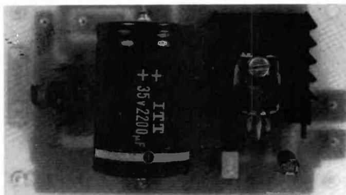
The 12V d.c. 1 amp stabilised power supply module which could also be used to power any project requiring 12V d.c.
