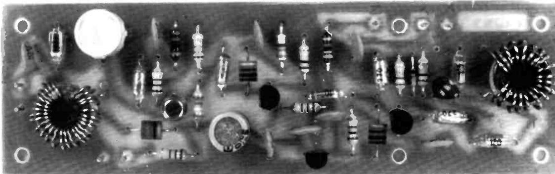
The completed 20m v.f.o. board. A dual varicap diode is fitted for tuning purposes.
