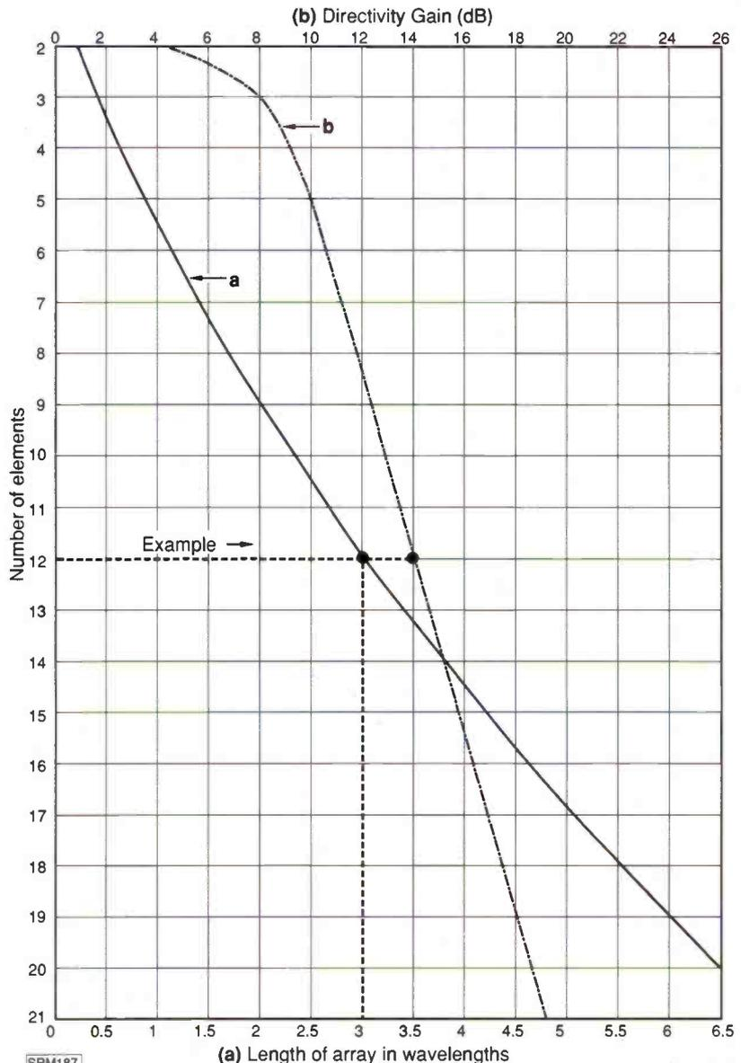
Fig. 9.2. Long Yagi data: directivity gain v antenna length and number of elements.
