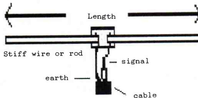
Fig 1: A cost-cutting dipole for satellite use
