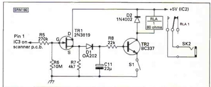
Fig. 3: Circuit of the automatic tape switch.
