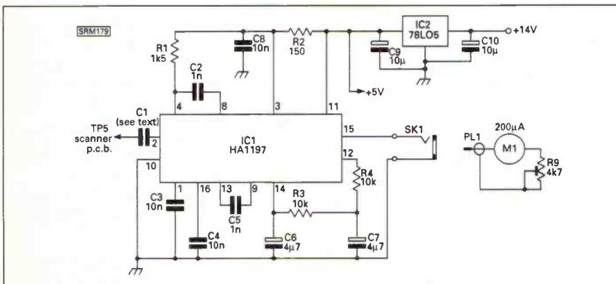
Fig. 1: The S-meter drive circuit.
