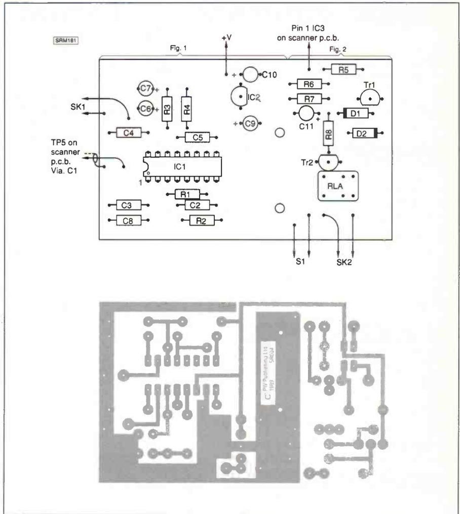
Fig. 2: Full-size p.c.b. track plan and component layout for the modifications described.
