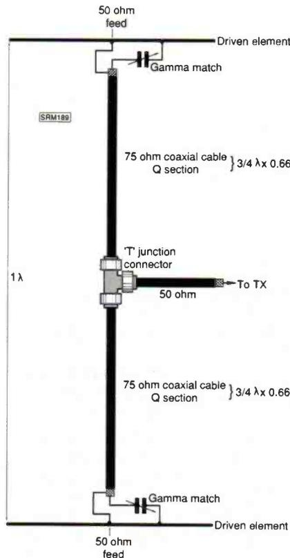
Fig. 9.4. One method of feeding two stacked Yagi beams. (Acknowledgements to *Practical Wireless*)
