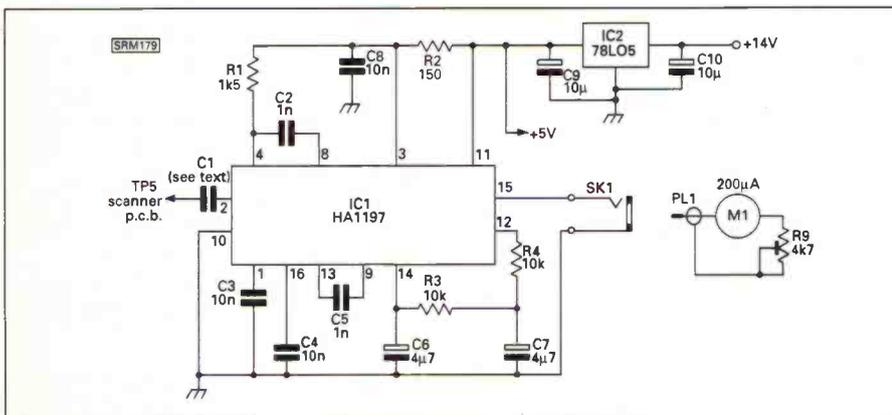
Fig. 1: The S-meter drive circuit.
