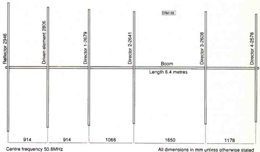
Fig. 9.3. Typical dimensions for a long Yagi parasitic beam antenna for the 50MHz band.
