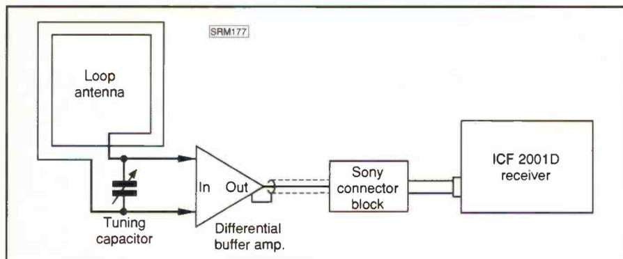
Fig. 2.2: Use of tuned loop antenna.
