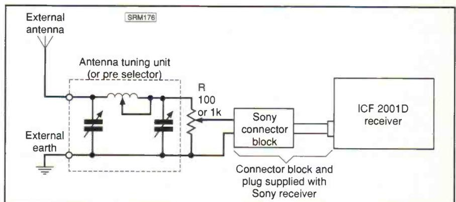
Fig 2.1: The use of preselection and attenuation.
