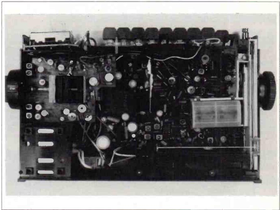
generally well made. The p.c.b. was made of s.r.p.b. board as opposed to the more common glassfibre, but it was well supported so shouldn't give any problems. The speaker was a 150 x 70mm elliptical type which contributed significantly to the final sound quality.
