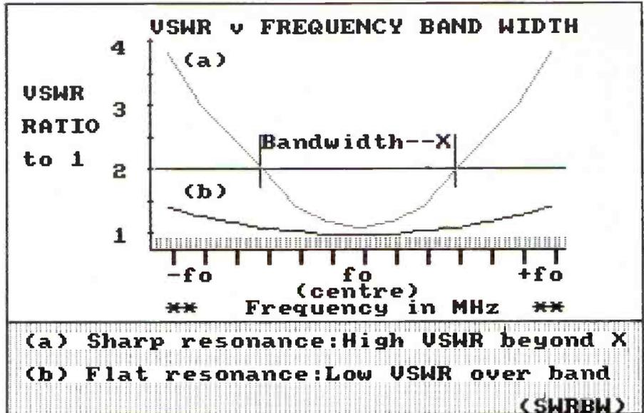
Fig. 9.1. Operational bandwidth versus v.s.w.r. See text for further details.
