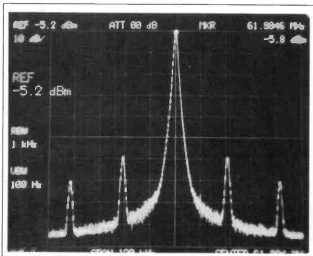
Fig. 3.1: Unmodified local oscillator spectrum. Scales: Horizontal 12kHz/div. Vertical 10dB/div. RX tuned to 6.15MHz; v.c.o. 61.995MHz.
