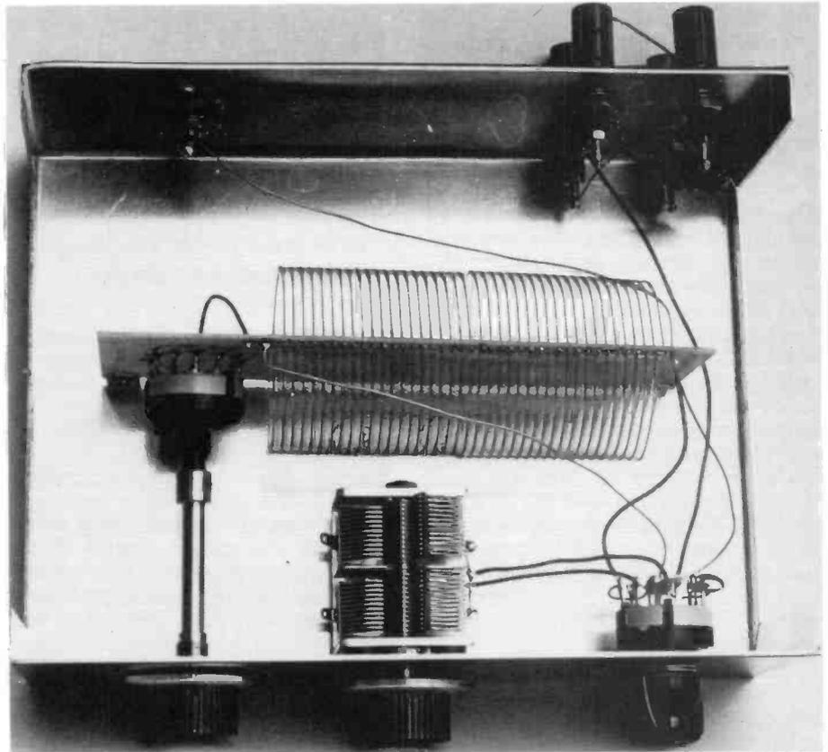
coped well with both antennas at all frequencies from 3 to 30MHz. My chief interest is the amateur bands but I used it with my general coverage receiver on all the main broadcast bands and it worked well. I also tried the TU1 with my double antenna which has a balanced twin feeder. With the balun in the circuit, it tuned every amateur band from 3.5 to 30MHz. I also used it with a low power (5 watt) transceiver on 3.5 and 14MHz and had several successful contacts on both bands.
