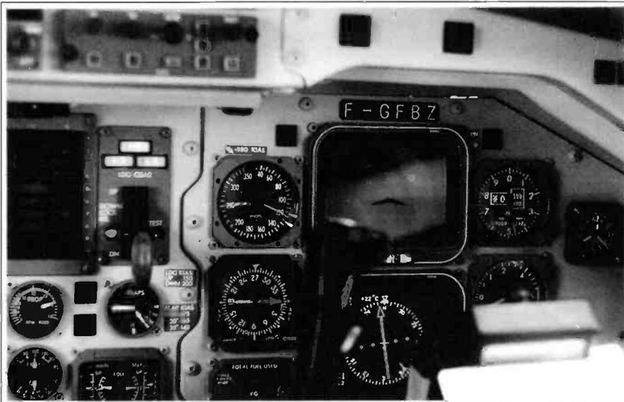
Saab 340A F-GFBZ (083) of Brit Air approaching Runway 26L at Gatwick. Descending through 60ft on the QFE 1008mb, threshold speed 115kts almost achieved. Wind 295° 12kts hence drift correction as seen on the h.s.i. (i.l.s. is tuned in). Gear down and locked. *Photo Godfrey Manning.*
