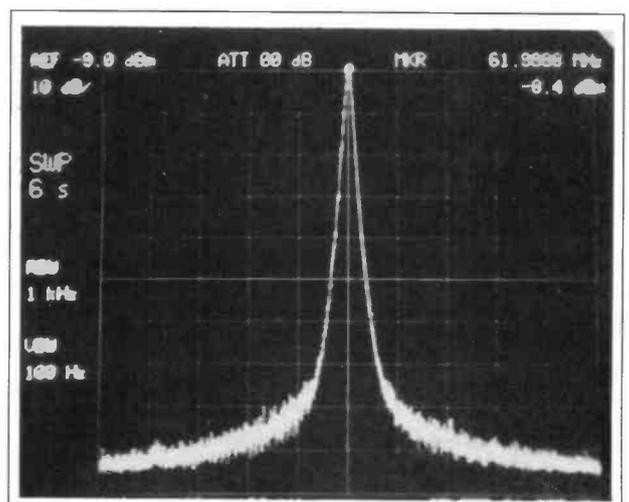
Fig. 3.2: The modified local oscillator spectrum. Scales: Horizontal 12kHz/div. Vertical 10dB/div. RX tuned to 6.15MHz; v.c.o. 61.995MHz.
