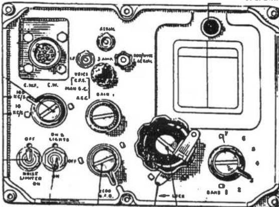
EX-MILITARY COMMUNICATIONS RECEIVER R210. Frequency 2 to 16MHz in 7 switched bands AM, CW, SSB, FCo, Aerial inputs 80ohm balanced line, long wire or whip, CW filter, BFO, Noise blanker, complete with 240 volt AC power pack, loudspeaker, headphone jack and pair of lightweight headphones.
