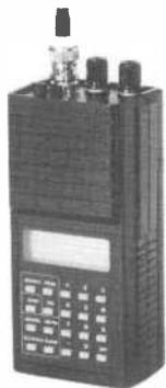
The established favourite hand held scanner from AOR is the AR-800E. This mighty midget covers 75-105, 118-174, 406-495, and 830-950MHz, and you can have AM or FM reception on any frequency in the tuning range. 20 memories, scanning, frequency searching, all the facilities you need, and it comes complete with rechargeable batteries, mains charger, and flexy aerial for an attractive price of only £199.
