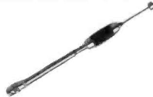
Extends the range of portable scanners. 9-sections, centre loaded. Frequency coverage 25–1300MHz. Connector is BNC.
