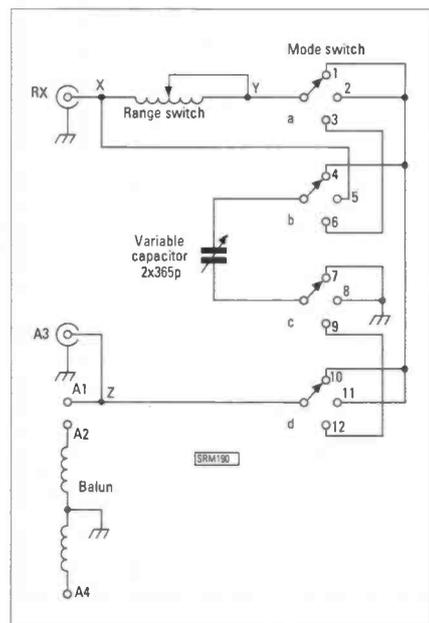
Fig. 1: Circuit diagram of the a.t.u.
