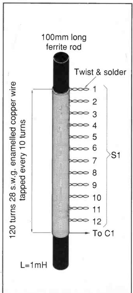
Fig. 2: Coil winding details for the m.w. version of the booster.
