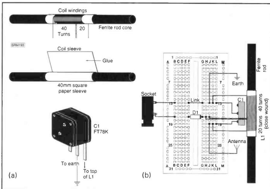
Fig. 2.2: (a) Coil winding and tuning capacitor details. (b) Layout and wiring diagram of the complete crystal set.
