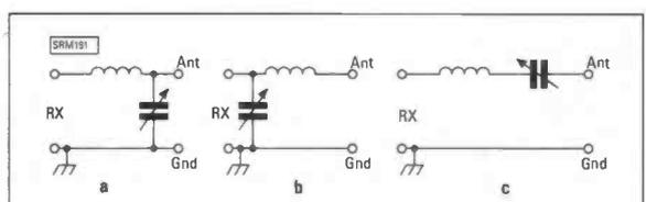
circuit which may be used in some cases of wide impedance mismatches between antenna and receiver. In most cases, the configuration in Fig. 2(a) will be required by the short wave listener.
