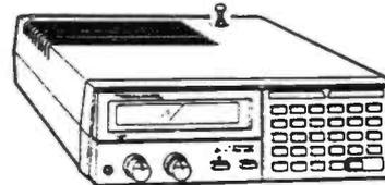
A Direct Entry Scanner with 200 memories which covers 68–88MHz, 108–136MHz (AM), 136.005–174MHz, 380–512 AND 806–960MHz.
