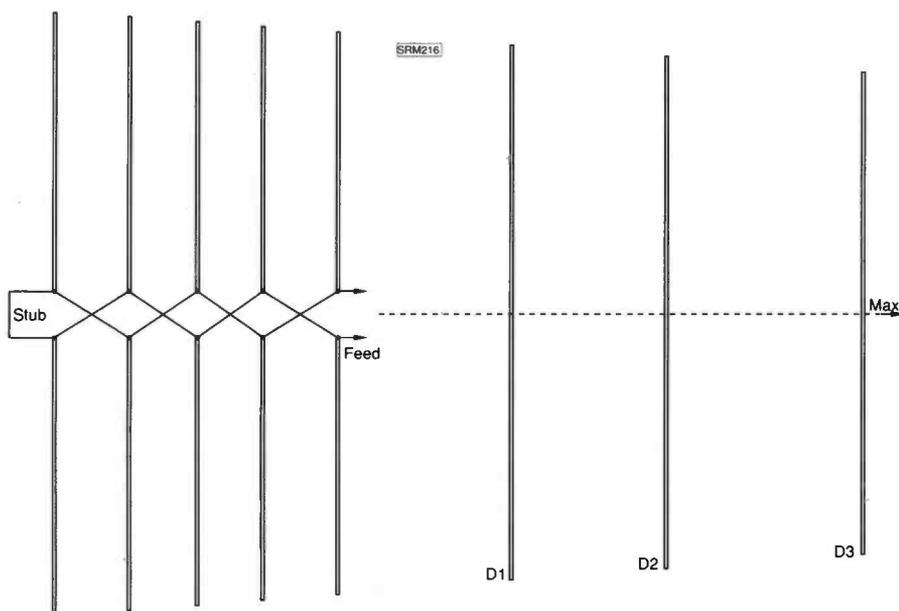
Fig.11.2: Arrangement of the log-periodic 'bandpass' antenna; D1, 2, 3 and 4 are passive elements (directors).
