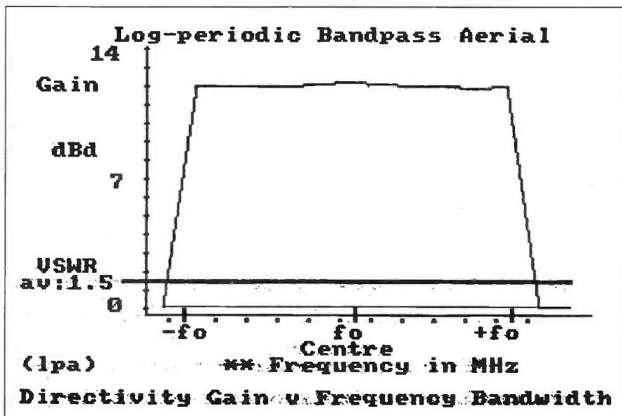
Fig.11.3: Directivity gain v. frequency response of the log-periodic bandpass antenna shown in Fig.11.2.
