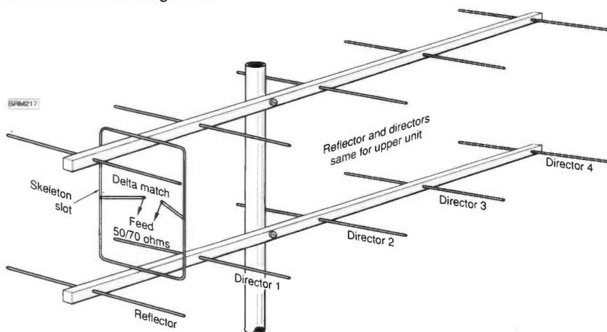
Fig.11.4: A 6-over-6 skeleton slot v.h.f. beam, see text.
