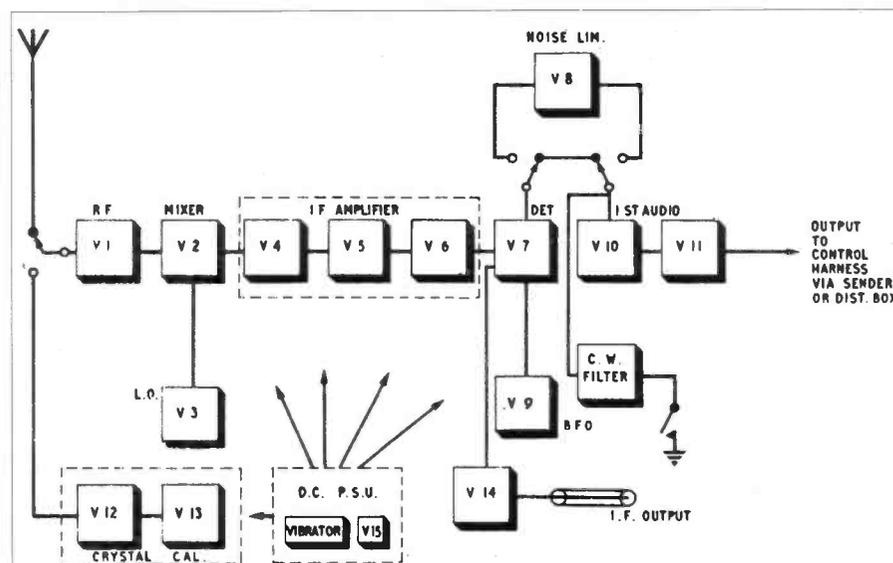
Fig. 1.1: Block diagram of the R210 receiver.
