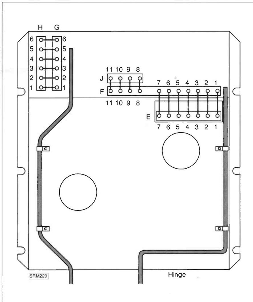
Fig. 1.2: The positions of the various tag-strips on the swing-out p.s.u. chassis.
