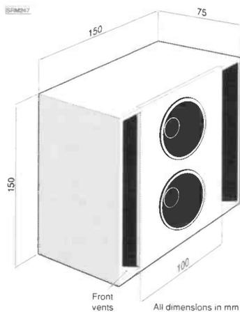
Fig. 8. Suggested loudspeaker enclosure design to provide tone correction. Note the side vents to reduce low-frequency response by cancellation. The whole front of the enclosure could be covered with a light speaker cloth.
