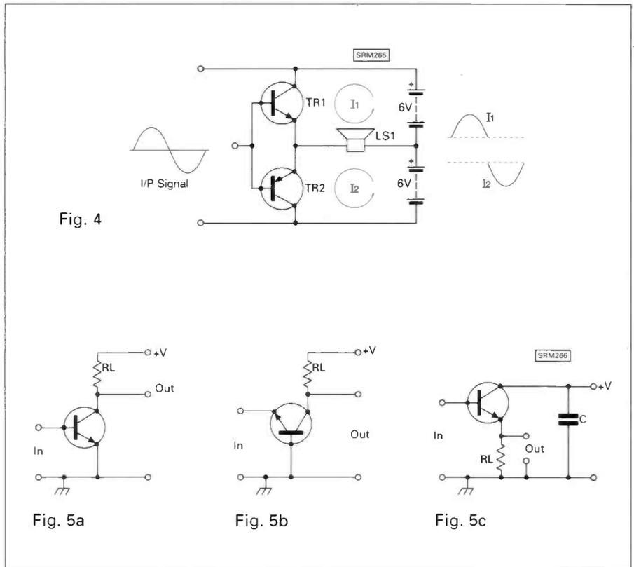
employed a complementary pair of low power (*nnp/pnp*) transistors in the driver stage, but a matched pair of *nnp* power transistors were operated as a single-ended push-pull output stage in Class B. When very high power levels of audio are required it may still be necessary to construct the amplifier along those lines:
