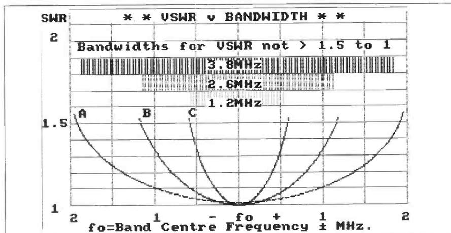
Fig. 14.1: Typical v.s.w.r. versus bandwidth of an antenna relative to centre frequency,  $f_0$ .
