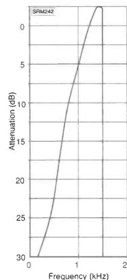
Fig. 3. Required response of a tone-correction circuit to obtain the ideal audio response for s.s.b. reception with the filter characteristics shown in Fig. 2.
