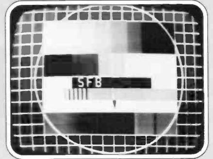
Fig. 3: The FuBK pattern is an alternative electronic test card used by many television services around the world. It was originally designed in West Germany and is now used on satellite television services.
