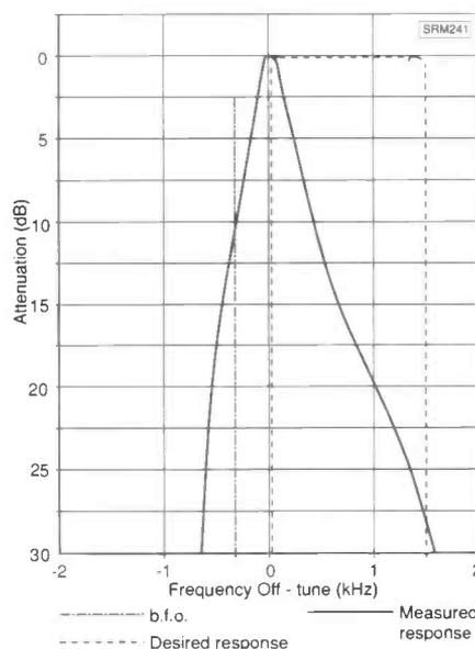
Fig. 2. Measured i.f. response of an Eddystone 730/4 receiver with the crystal gate switched in and the phasing control in the position for u.s.b. reception. The dashed curve shows the ideal frequency response for selective s.s.b. reception with the b.f.o. at the frequency indicated.
