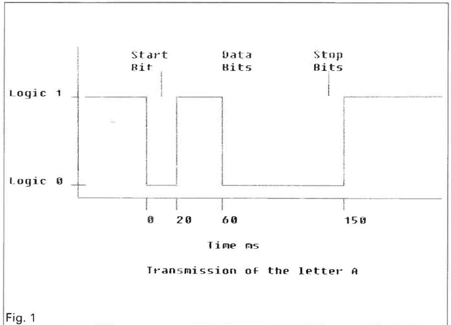
that they all stay in the right order, so that we can reverse the process at the other end. So this is the basis of serial data. Before we move on I ought to make one point clear about the ITA2 code. Although I have talked about computers operating with eight bit binary numbers, the ITA2 code is actually a five bit code. This might seem a little confusing, but really all it means is that the highest three of the eight bits used in the computer are ignored.
