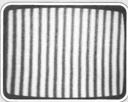
Fig. 9: The electronically generated, vertical stripes, test pattern is radiated on rare occasions by Russia and Spain. The number of stripes can vary.
