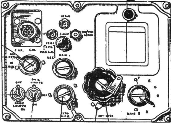
EX-MILITARY COMMUNICATIONS RECEIVER R210. Frequency 2 to 16MHz in 7 switched bands AM, CW, SSB, FCo, Aerial inputs 80ohm balanced line, long wire or whip, CW filter, BFO, Noise blanker, complete with 240 volt AC power pack, loudspeaker, headphone jack and pair of lightweight headphones.
