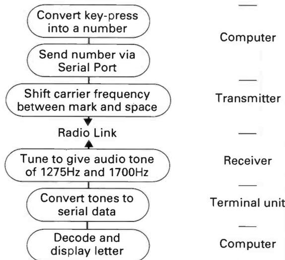
Fig. 2.5: RTTY system flow chart.
