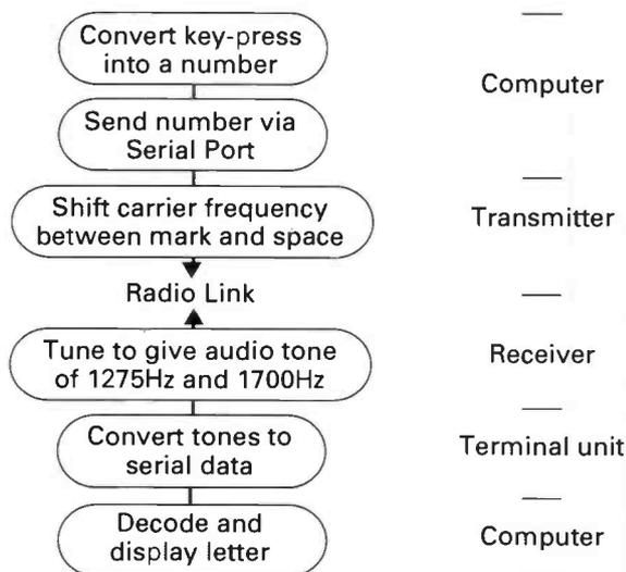
Fig. 2.5: RTTY system flow chart.
