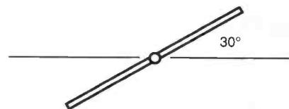
Fig. 3: The Lindenblad antenna viewed from above showing connections for right-hand polarisation.
