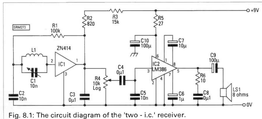
Fig. 8.1: The circuit diagram of the 'two - i.c.' receiver.
