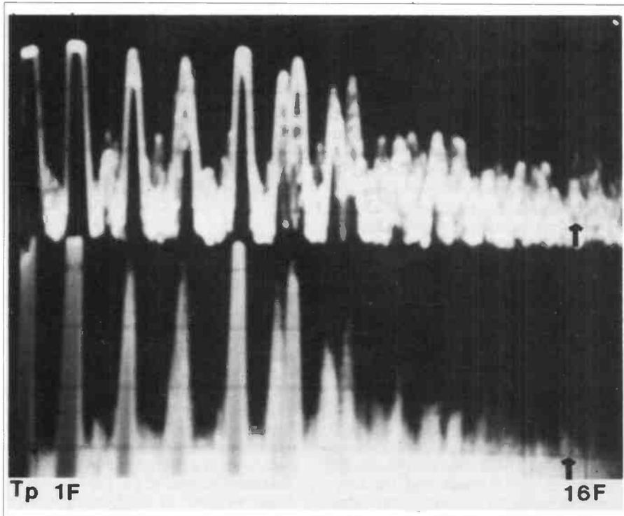
Fig. 1: (Upper trace) Rectified pulse signals. (Lower trace) Tp - transmitted pulse 0.5ms duration; p.r.f. = 35p.p.s.; 1F - primary signal from F region; 16F - sixteenth multiple echo.
