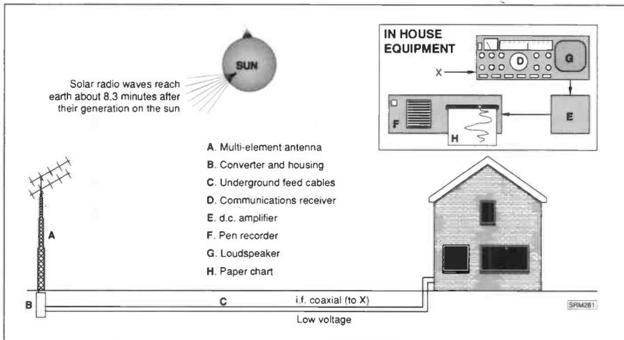
Fig. 1.1: The 'spreadout' superhet radio telescope.
