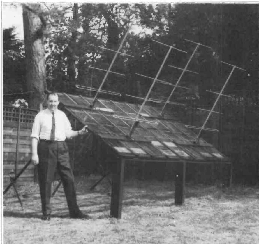
Ron Ham with the 136MHz solar telescope antenna array in his garden in 1968.
