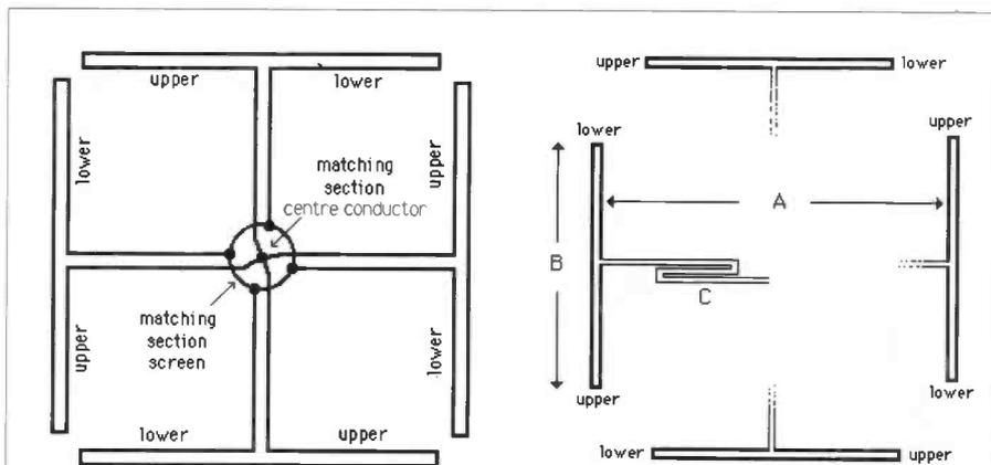
Fig. 1: The layout of the Lindenblad antenna. The dimensions A, B and C are found from Table 1.
