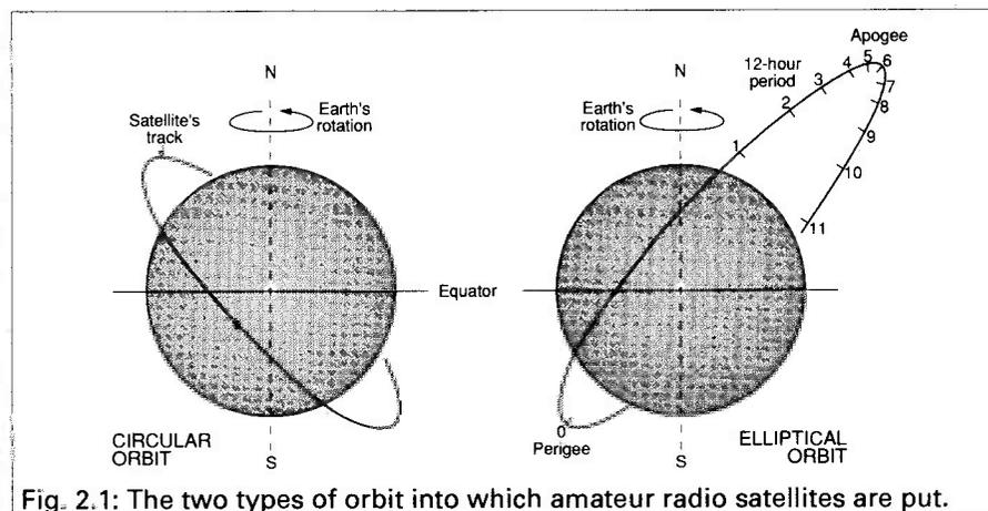
**Fig. 2.1: The two types of orbit into which amateur radio satellites are put.**
