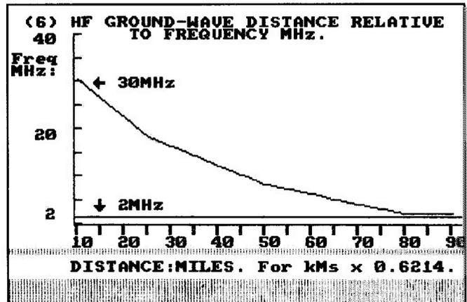
(6) Approximate 'ground wave' propagation distance versus frequency of operation up to 30MHz. Note that at 2MHz the curve flattens out at about 80km. At lower frequencies (medium wave band) the distance may not extend to much more than 100km although this increases as the frequencies become lower still (long wave band).
