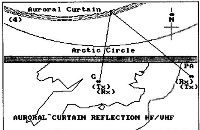
(4) The 'Auroral Curtains' that form at the extremes of the Northern and Southern hemispheres can become ionised in the same way as an ionospheric region and can, therefore, reflect radio waves at both h.f. and v.h.f. An actual v.h.f. path is shown here which allowed a two-way radio contact to be carried out between central England (G) and Holland (PA).
