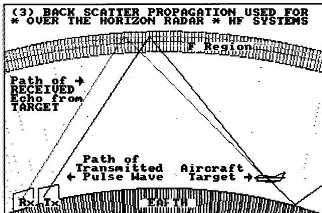
(3) In which 'scatter' propagation via the F region is used to advantage. This is the 'back scatter' mode employed by the US Defense Department for the detection of high or low flying aircraft, or guided missiles, at very long ranges, known as 'over the horizon radar (OTHR)'. (*Practical Wireless* August 83). An h.f. spectrum 'surface radar' system (this makes no use of the ionosphere) is now in operation in the UK.
