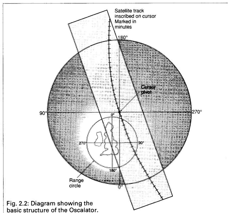
**Fig. 2.2: Diagram showing the basic structure of the Oscalator.**
