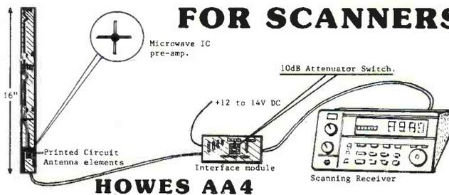
The new **HOWES AA4** Active antenna gives full coverage from 25 to 1300MHz. It is designed to be the ideal solution for those requiring a compact, broadband antenna for use with scanning receivers. The AA4 features advanced technology with a low noise microwave IC as the active element.
