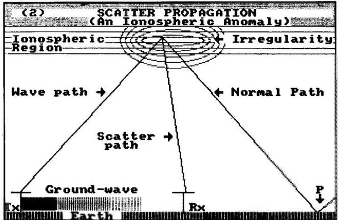
(2) Scatter propagation can occur in various ways and one is due to the occurrence of irregularity in an ionised region. A forward wave is refracted in the normal way but a patch of irregular ionisation can also refract the same wave at the same time, along a steeper, but still forward, path. Signals propagated this way are usually not very strong.
