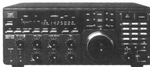
The NRD525 is a high class, general coverage receiver with expandability looking to the future. Combining traditional technology unique to JRC with the most advanced digital technology gives superb performance whilst remaining extremely easy to use. The NRD525 covers 90kHz-34MHz and with an optional VHF/UHF converter also covers 34-80, 114-174 and 423-456MHz. Modes of operation CW, SSB (USB/LSB), AM, FM and RTTY with optional demodulator.
