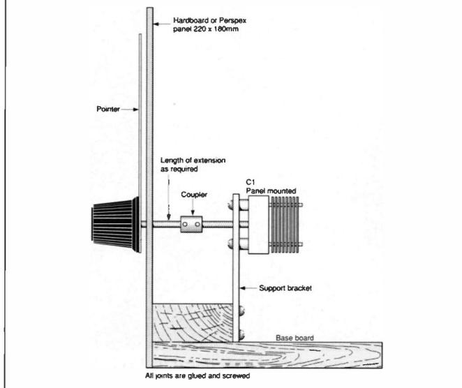
length of 1.5mm 'twain & earth' lighting cable is ideal). Place in position and wind three turns tightly round the shaft using a pair of pliers. The pointer can now be soldered or glued to the shaft.
