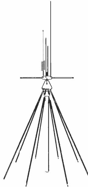
Most discones only have horizontal elements and this is the reason that they are not ideal for use with a scanner. Most of the transmissions that you are likely to receive on your scanner are transmitted from vertically polarised antennas. The Sky Scan V1300 discone has both vertical and horizontal elements for maximum reception. The V1300 is constructed from best quality stainless steel and aluminium and comes complete with mounting pole. Designed and built for use with scanners.
