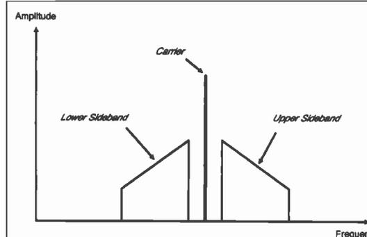
Fig. 1: An a.m. signal.
