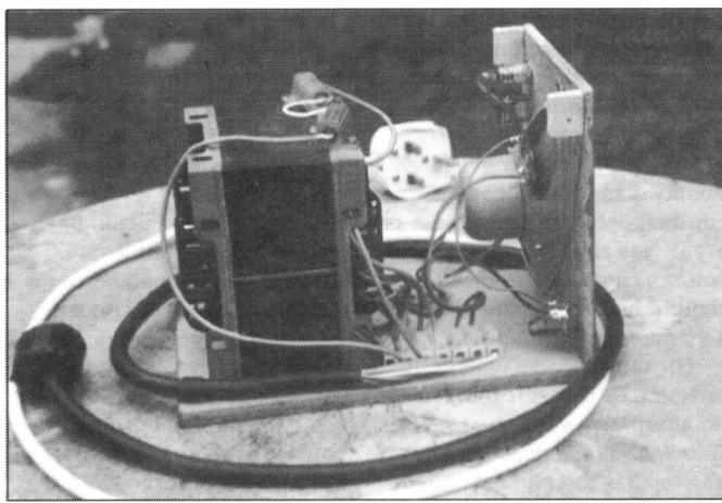
*The power supply and external loudspeaker unit.*
