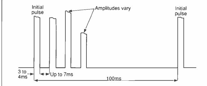
**Fig. 2: Four-pulse Russian 'Woodpecker' transmission, unmodulated sequence (see text).**
