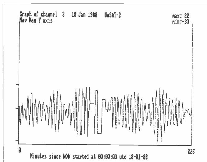
Fig. 2: Graphical plot of the navigation magnetotorque Y-axis during part of an orbit in January 1988.
