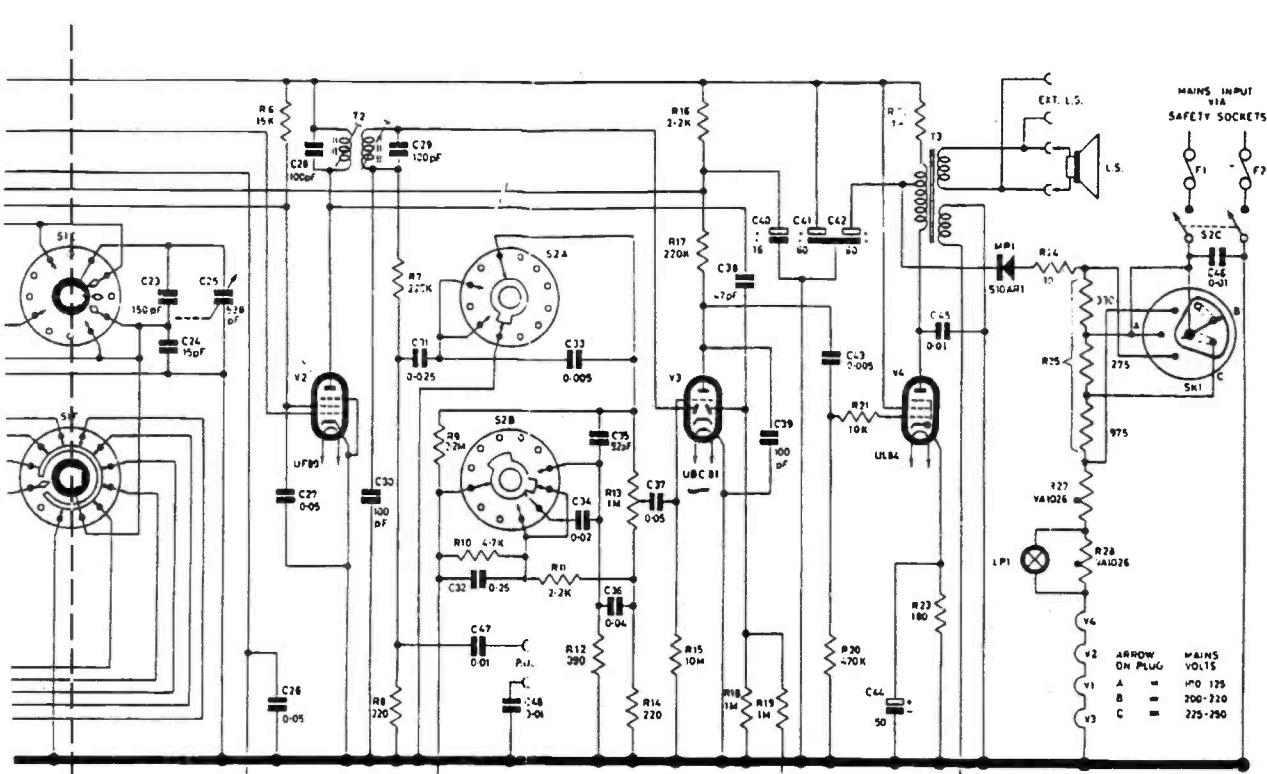
*The circuit diagram of the Pye 3017A (Export) radio taken from the service manual. The diagram has been split into two, about the vertical broken lines, to enable it to be fitted onto this page.*
