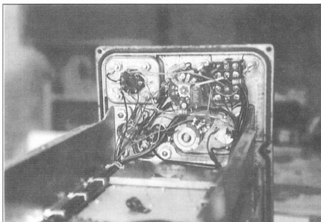
The inside of the R210 showing the back of the front panel with the new Octal socket and its wiring.
