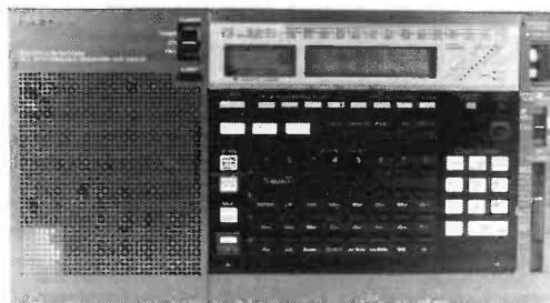
The **ICFPRO80** is a handheld professional receiver with air band capability and an 8-way tuning system. Frequency coverage 150kHz-108MHz and 115.15kHz to 223MHz with FRQ 80 frequency converter.
