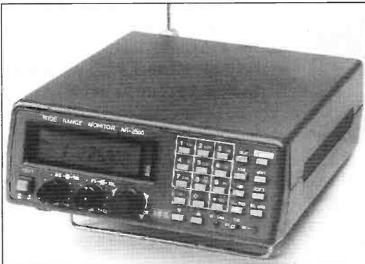
**AR2500** Base/mobile scanning receiver featuring coverage from shortwave to microwaves 500kHz – 1500MHz with no gaps. All mode AM, FM (narrow), FM (wide), and built-in BFO for USB, LSB, CW. An 'Elephant' memory can store 1984 spot frequencies and 16 search groups. The memory is permanent using an EEPROM (but can be overwritten). Computer control is available via the RS232 port on the back panel. The AR2500 is operated from 13.8V DC. Performance and flexibility at an affordable price.
