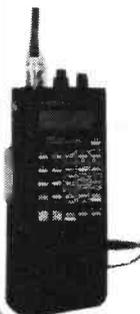
The **Bearcat 200XLT** is the cream of the Bearcat handheld scanner range. With 200 memory channels and simple operation these are proving very popular. Freq. coverage 66-88, 118-174, 406-512 and 806-956MHz.
