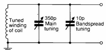
(b): Adding bandspreading by electrical means.
