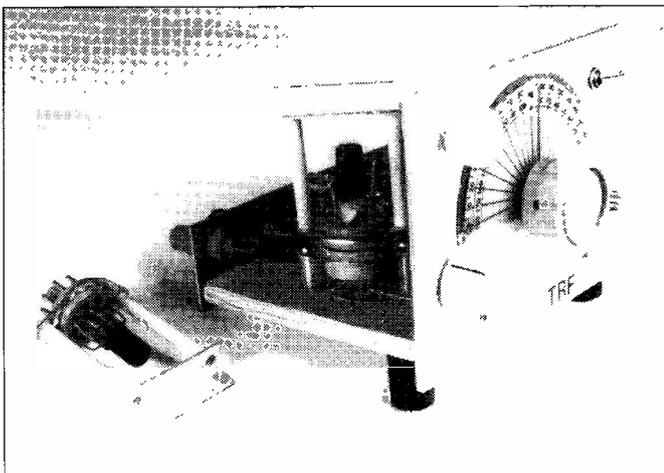
Two views of prototype SWM t.r.f. receiver built by George Dobbs G3RJV, showing the simple construction and plug-in coil.
