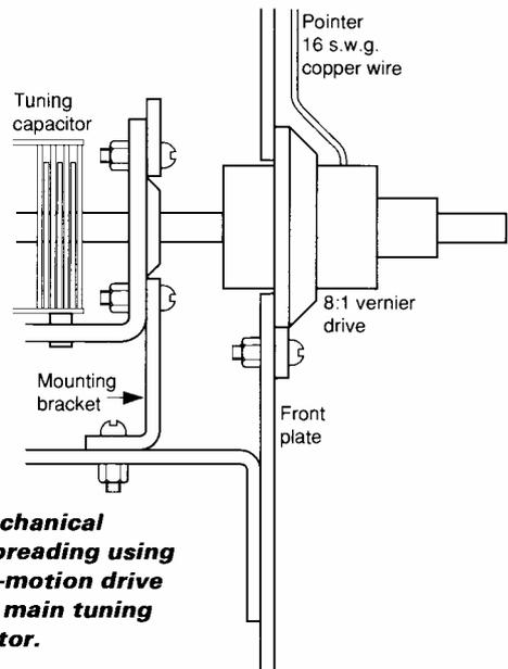
(a): Mechanical bandspreading using a slow-motion drive on the main tuning capacitor.
