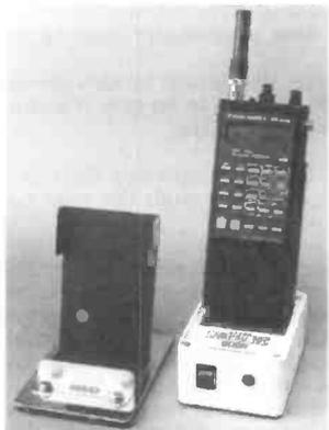
2. **JIM BH-A3.** Universal base stand for handheld scanners-transceivers etc. convenient, safe support of radio. Adjustable front stop. Heavy duty chromed base. Bracket for BNC socket for base antenna connection. **PRICE £9.95.**
