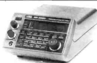
AOR AR3000, Unique top of the range wide band scanning receiver. All mode AM, FM-N, FM-W, USB, LSB, CW. Frequency coverage is 100kHz-2036MHz with no gaps. Supplied with telescopic aerial, 13.8V DC lead, and AC power supply. £765
