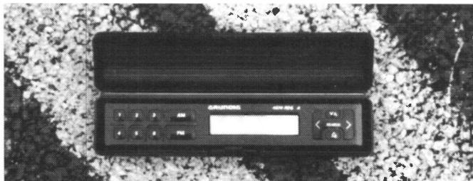
The front panel of the WKC 4870 RDS car radio can be removed for added security.
