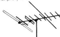
Complete with folded dipoles for both Band 1 and Band3 for optimum performance. Covers Band 1 (47-70MHz) at 3.5dB gain. Band 3 (175-230MHz) at 8dB gain.
