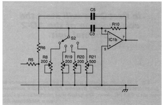
**Fig. 1.4: Modifications to the circuit of the AD-2 terminal unit to add extra shifts and variable shift.**
