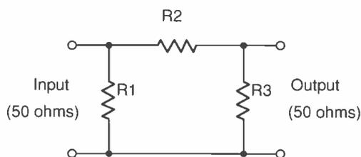
**Fig. 1: Basic Pi section attenuator. For resistor values see Table 1.**
