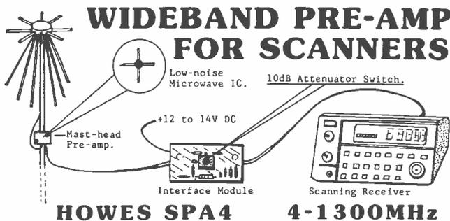
The **HOWES SPA4** wide-band pre-amplifier is designed to add extra gain to passive antennas (discone, nested dipoles etc.). The low noise combined with at least 15dB of gain over the whole frequency range overcomes the losses in the antenna's down lead, and adds extra sensitivity to the scanning receiver.
