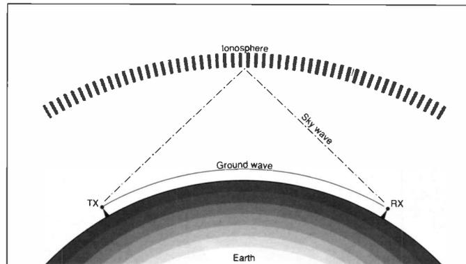
Fig. 1: Multi-path propagation.
