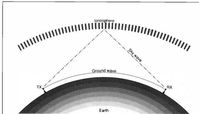
Fig. 1: Multi-path propagation.
