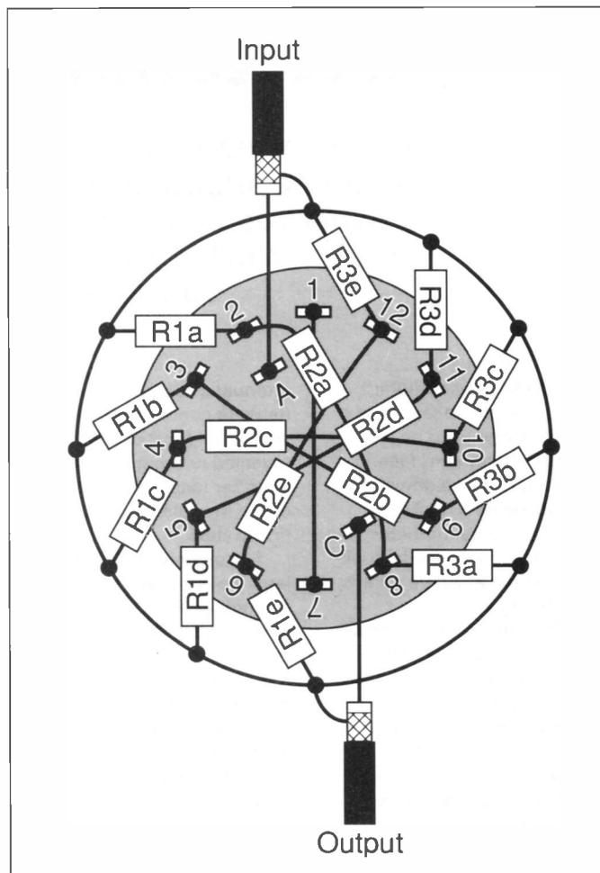
**Fig. 2: The resistor positioning and connections for the attenuator switch.**
