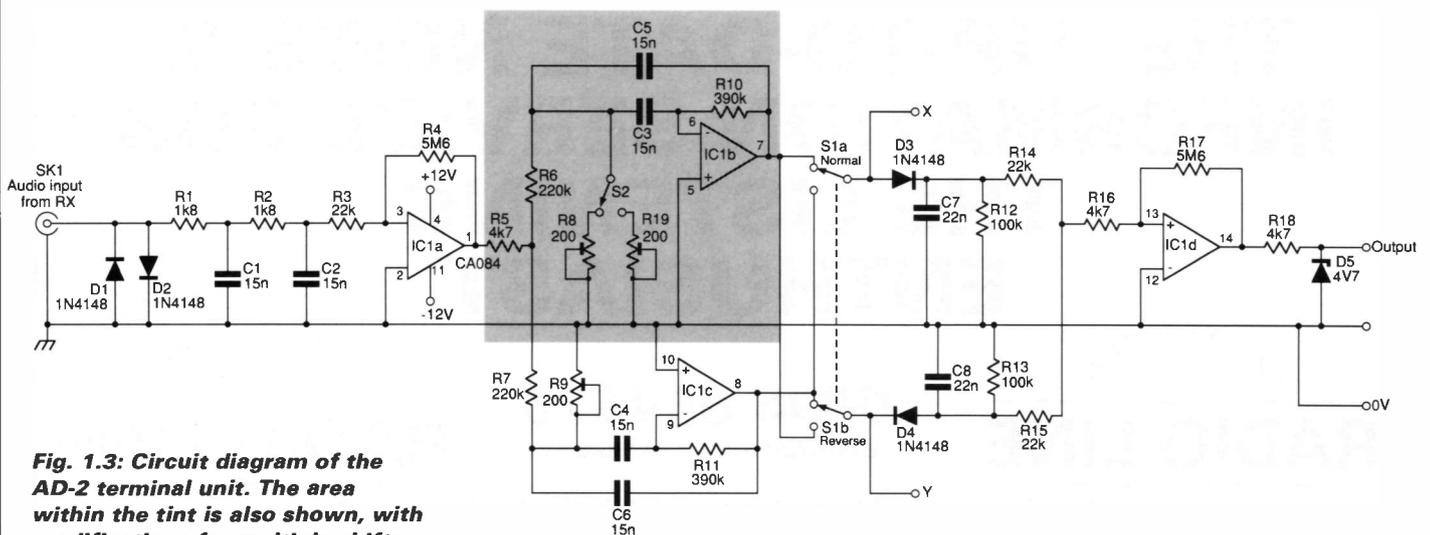
**Fig. 1.3: Circuit diagram of the AD-2 terminal unit. The area within the tint is also shown, with modifications for multiple shifts, in Fig. 1.3.**
