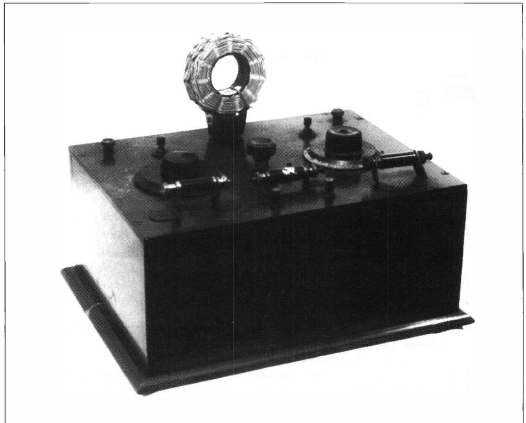
**A luxurious home-built crystal set having a choice of three different crystals and other refinements. On top can be seen the long wave '5XX' coil that was switched in to receive Daventry. Sixty-six years later the set still works perfectly.**
