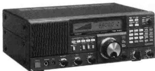
The **FRG8800** HF communications receiver. A better way to listen to the world. Continuous coverage from 0.15-30MHz optional module for VHF coverage from 118 to 174MHz. SSB, CW, AM & FM modes. Direct frequency entry keyboard.
