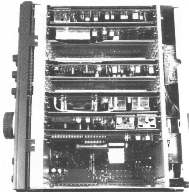
**A view inside the NRD-535 showing how much has been fitted into the receiver.**
