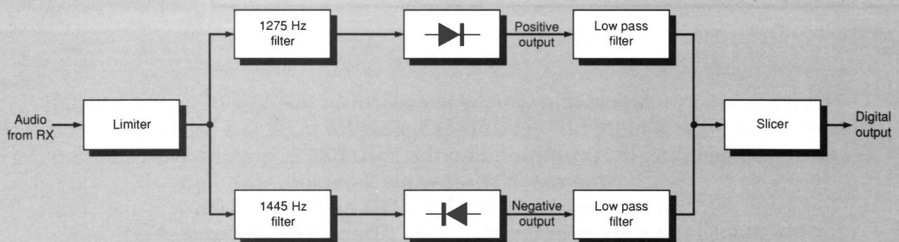
**Fig. 1.1: Block diagram of a basic receive-only terminal unit.**
