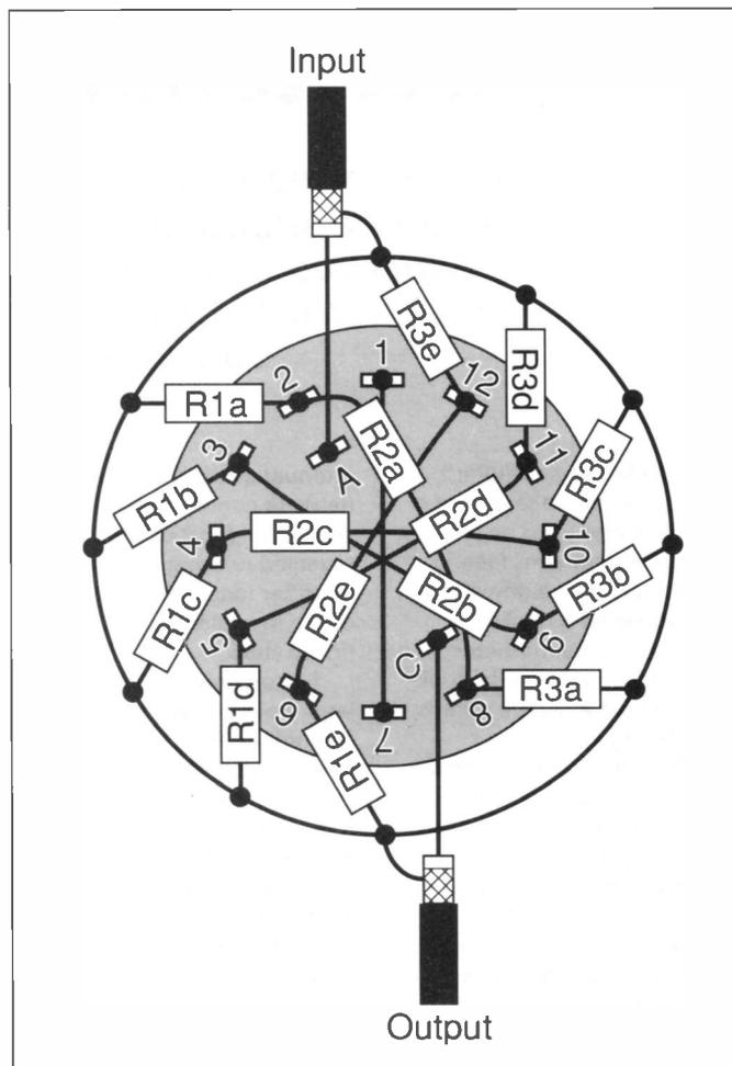
Fig. 2: The resistor positioning and connections for the attenuator switch.
