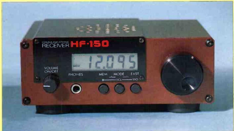
**Aerial inputs:** 600 ohms, 50 ohms & Hi-Z Whip
