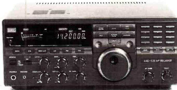
There are 200 memory channels, each of which stores, frequency, mode, bandwidth, attenuator and AGC settings, comprehensive frequency sweep facilities and no less than 16 different functions which can be programmed from the front panel by the user.
