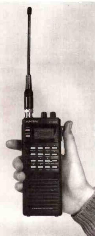
The VT-225 is a civil and military airband receiver, covering 108-142MHz v.h.f. and 222-391MHz u.h.f. Its main features are:
