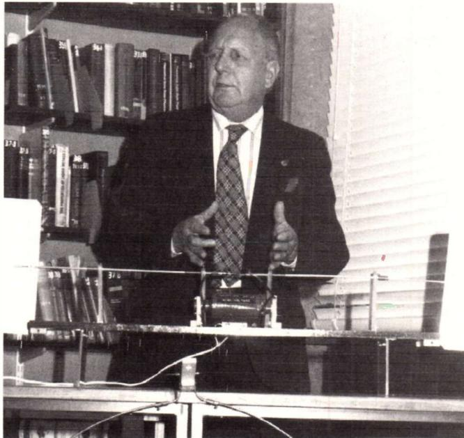
**F.C. Judd A Inst E, G2BCX demonstrates his working replica of the apparatus used by Heinrich Hertz for the 'discovery of wireless waves' experiment in 1880. The demonstration took place at the University of East Anglia, School of Physics and Fred later presented the replica apparatus to the School.**
