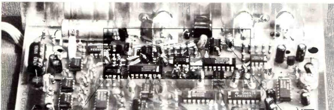
*This annotated photograph shows the four capacitors that are to be changed for 3.3nF.*
