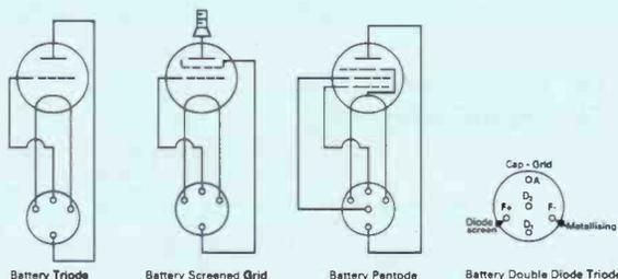
Fig. 1: Connections for 4-pin, 2V, battery valves. Taken from *Radio Receiver Servicing* by E.G.J. Lewis 1945.
