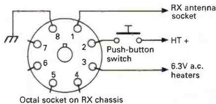
**Fig. 3: Octal socket connections.**
