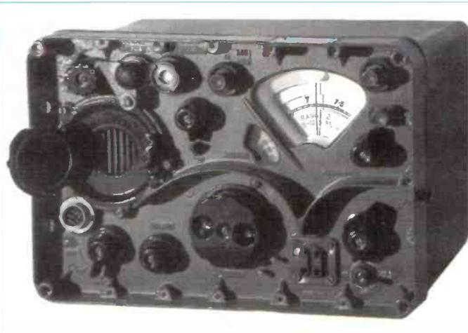
does not require interconnection to any other units to perform as a receiver. It appears in a number of Marks, which differ principally in the power source they can use, early models requiring 6V d.c. input while later versions can accommodate 12V or 24V d.c. or 110/240V a.c., selected from a panel switch. There are other, less obvious, minor differences between models.
