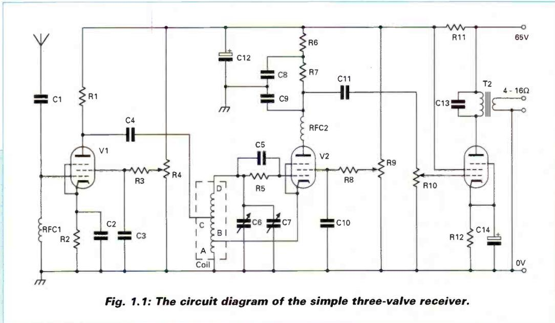
Fig. 1.1: The circuit diagram of the simple three-valve receiver.
