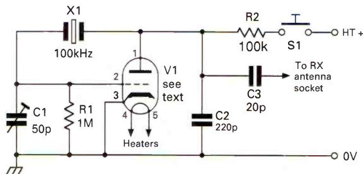
Fig. 1: Simple, basic 100kHz crystal oscillator.
