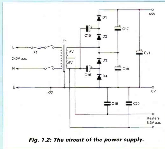
Fig. 1.2: The circuit of the power supply.
