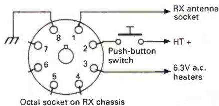
**Fig. 3: Octal socket connections.**
