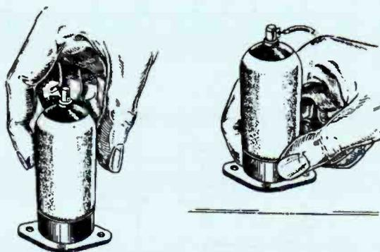
Fig. 2: The wrong way to remove a valve is shown on the left. The correct way, by gripping the valve's base, is shown in the right. Taken from *Everyman's Wireless Book* by F.J. Camm.
