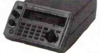
This receiver can only be described as the *smallest high performance receiver*, with nearly every possible facility available. Just look at the spec: AM, FM, FM-W, USB, LSB, CW, on all frequencies. Continuous tuning from 100kHz - 2036MHz, full remote control via RS232 port, tuning rate as low as 50Hz, 400 memory channels. Size dimensions 138x80x200 (WxHxD) (mm).
