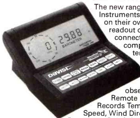
The new range of Davis Instruments can be used on their own with an LCD readout or can be connected to a computer for long term data logging. 32K inbuilt memory (stores up to 120 days observations).
