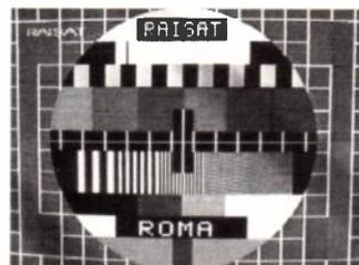
Fig. 2: RAISAT TV seen over the Olympus satellite 12.169GHz at 19°W.
