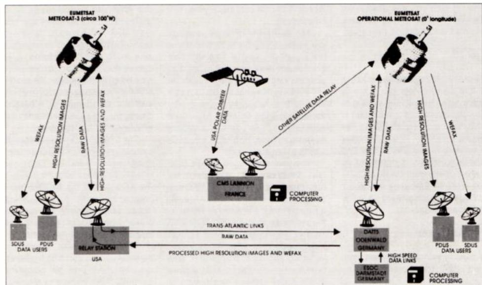
Fig. 1: The Atlantic Data Coverage Extension; courtesy EUMETSAT
