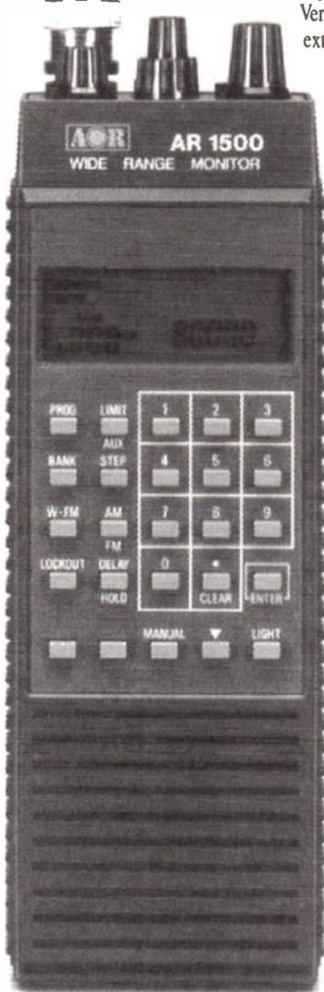
Versatility is excellent. The AR1500 may be powered from its internal NiCad pack, spare dry batteries may be carried for extended operation and used with the dry battery case. The set may also be plugged directly into the cigar lighter socket of a motor vehicle (external input range 11 - 18V DC).
