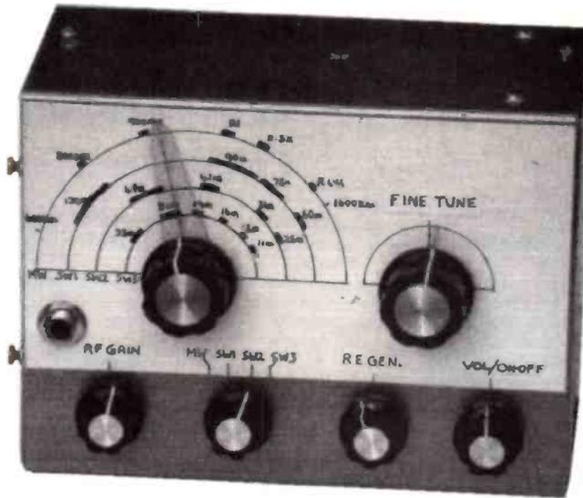
Start by temporarily fixing the blank 'dial' in the correct position on the front panel. Then put the main pointer on the shaft of C6 and inserting a fine tip marker pen through suitably drilled holes in the pointer draw the four scales on the dial.
