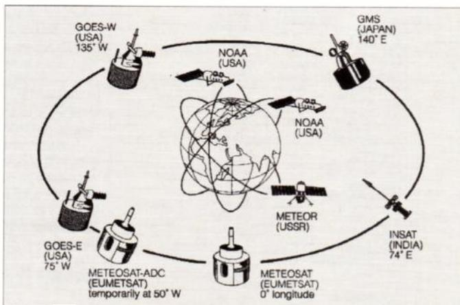
**Fig. 3: Global Meteorological Satellite System; courtesy EUMETSAT.**
