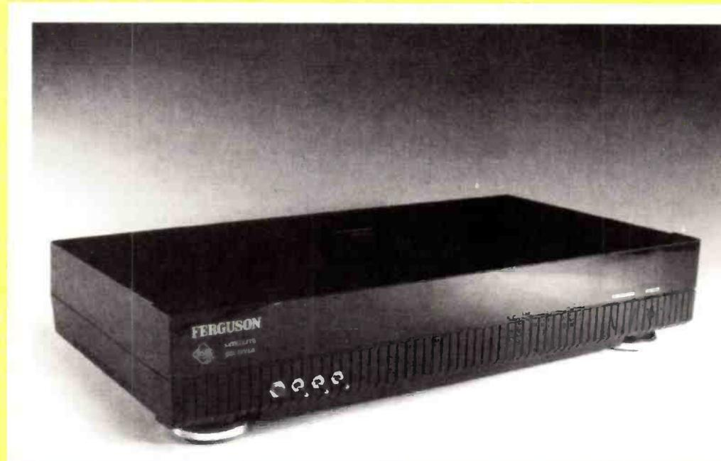
**The Ferguson SRB1 satellite receiver after conversion to receive D-MAC, D2-MAC and ASTRA PAL signals. The switches on the left of the front panel are the Reset push button, followed by the vertical/horizontal polarisation switch for ASTRA. The next switch along is the PAL/D-MAC selector switch followed by the D-MAC/D2-MAC switch. Labels identifying the switches and their functions have still to be fitted.**
