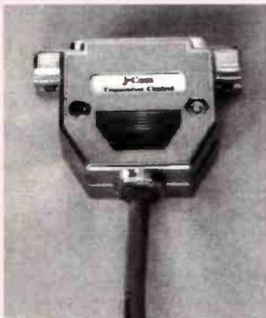
The j-Com interface cable requires no external power supply and draws just 3.5mA of power for the Icom and Yaesu models and 6mA for the Kenwood version. This small amount of power can be 'borrowed' directly from the computer's serial interface.
