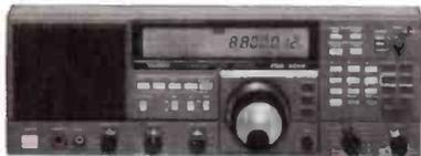
The **FRG8800** HF communications receiver. A better way to listen to the world. Continuous coverage from 0.15-30MHz optional module for VHF coverage from 118 to 174MHz. SSB, CW, AM & FM modes. Direct frequency entry keyboard.
