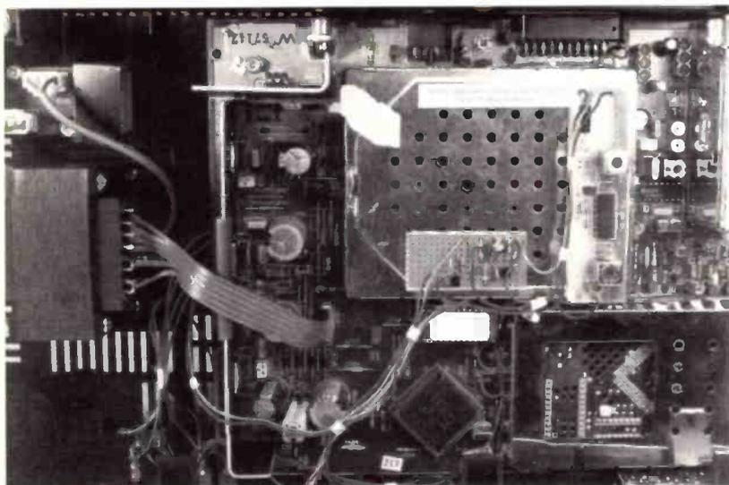
**The Ferguson SRB1 receiver with the top removed to show the Satellite Surplus D2-MAC and PAL conversions.**
