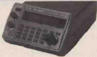
This receiver can only be described as the *smallest high performance receiver*, with nearly every possible facility available. Just look at the spec: AM, FM, FM-W, USB, LSB, CW, on all frequencies. Continuous tuning from 100kHz - 2036MHz, full remote control via RS232 port, tuning rate as low as 50Hz, 400 memory channels. Size dimensions 138x80x200 (WxHxD) (mm).
