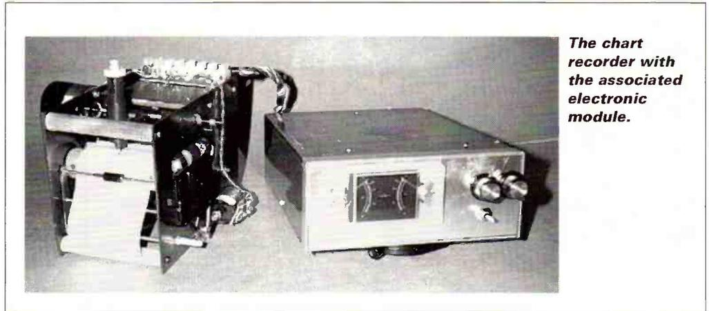
The chart recorder with the associated electronic module.
