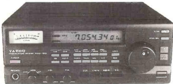
A new receiver from Yaesu has been a long time coming and the FRG100 sets a new standard from this manufacturer. Broadcast listeners may like the 6 and 4kHz bandwidths and the fifty memory channels will store both frequency and mode.
