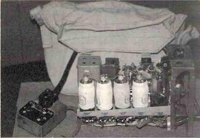
Fig. 2: The junction box and signals satchel of the WS-38.
