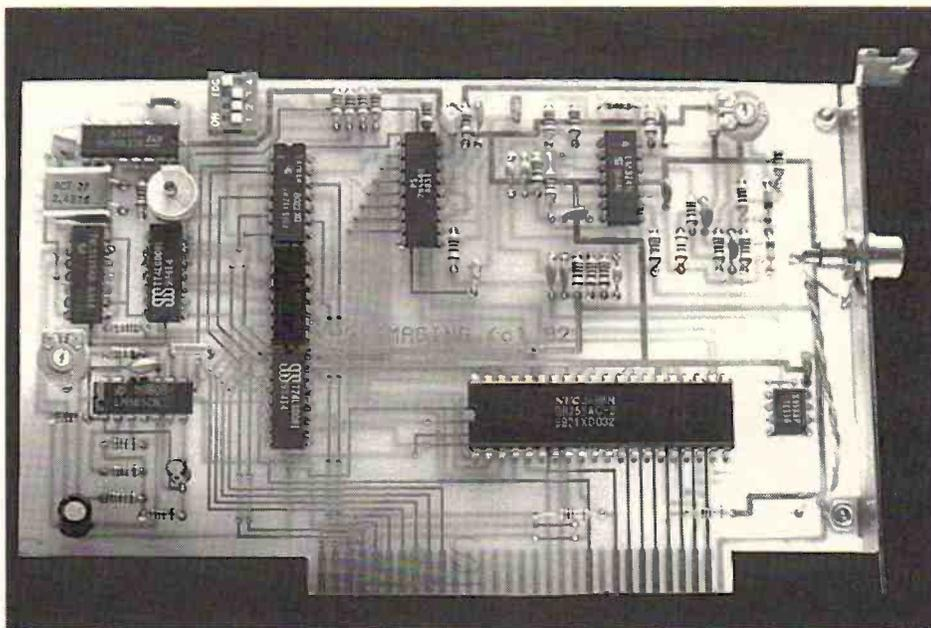
Fig 1: PC interface board - slots into a PC.
