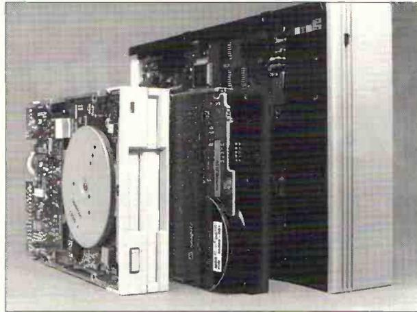
**Left to Right - 3.5in HD floppy disk drive, 120Mb 3.5in IDE hard disk drive and 20Mb 5.25in MFM hard disk drive**
