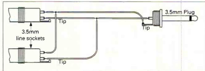
**Do-it-yourself version of a 3.5mm Y adaptor to break into the audio output of a receiver**
