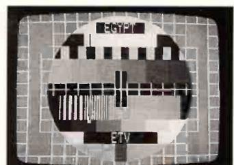
Fig. 6: The non-too strong PM5544 test card from Nile TV, Egypt on Eutelsat II F3 @ 16°E.
