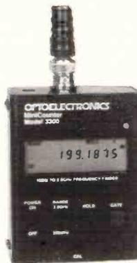
The problem with LED counters is that you can't see them in daylight and they consume massive amounts of current. The new M-3300 counter has LCD readout and is super sensitive. You get frequency hold, input filtering, ni-cads, AC charger and aerial.
