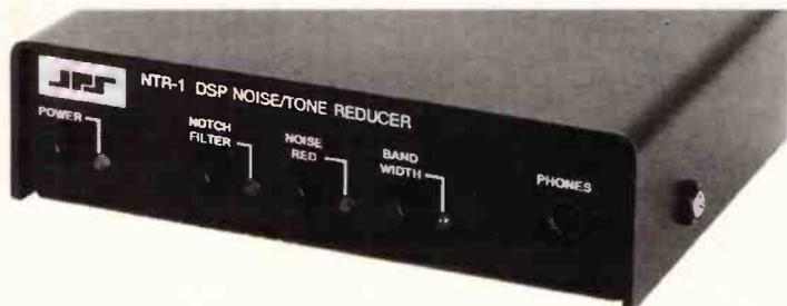
*The NTR1 is a sophisticated audio processing unit that uses Digital Signal Processing to provide superior operating characteristics to those attainable using analogue techniques. The unit takes the audio from the receiver and converts it into a digital bit stream, processes it and turns it back into an analogue signal.*
