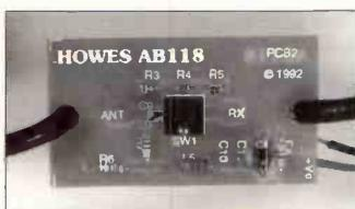
**Fig. 4: Power coupler and switched attenuator.**
