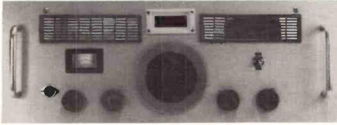
**Front View: Controls left to right – RF gain, AF gain, Squelch, S Meter zero. The large vents on either side of the frequency read-out assist with the air circulation and help to keep the receiver cool. At the left the DIN socket is for a tape recorder connection.**
