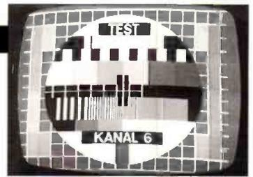
PM5544 test card via Eutelsat II F4 at 7°E - 11.163GHz vertical.
