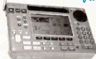
This top range portable gives you a complete station in a single package. On-board computer lets you store frequency and station name. You direct dial your frequency for high quality SSB or AM reception. Includes mains AC supply etc.
