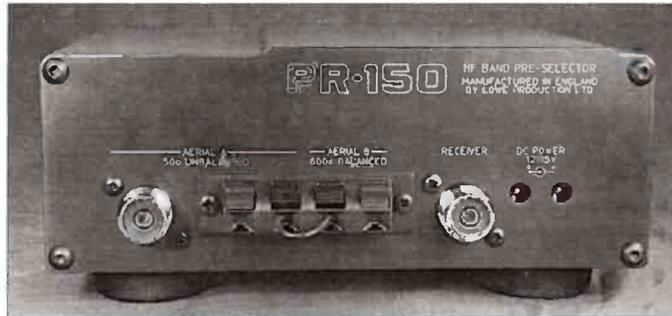
**Versatile antenna connectors and power out socket make this an extremely good mate for the Lowe Electronics HF-150 communications receiver.**
