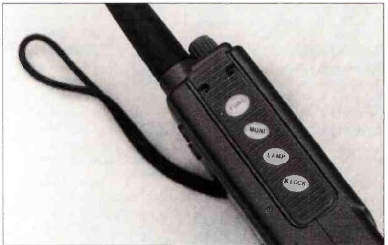
One could argue that once you've seen one scanner you've seen them all - not true. The AR8000 represents a significant step forward, particularly where portables are concerned. Not only does the AR8000 feature continuous coverage from 500kHz through to 1.9GHz, but it has tuning steps down to 50Hz, a 2.4kHz s.s.b. filter and true carrier reinsertion on s.s.b. and c.w. All this is supplemented by a versatile display system, twin v.f.o.s and 1000 programmable memories.
