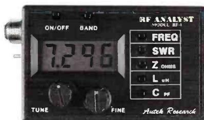
microprocessor, A/D converters and a low-distortion, levelled, sine-wave generator with a 4-digit frequency readout, continuously adjustable from 1.2 to 35MHz in five bands. It measures r.f. values of impedance (0-2000Ω), s.w.r. (1 to 15:1), Capacitance (0-9999pF) and Inductance (<0.04 to 300μH). The digital readout of all parameters is claimed to be unique in its price range.
