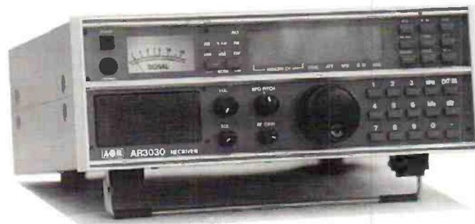
Following my review of the prototype receiver back in the January issue, I have now had the opportunity for a more detailed study of a standard production unit. The review model was completely standard except for the inclusion of the optional 500Hz Collins c.w. filter and an external power lead.
