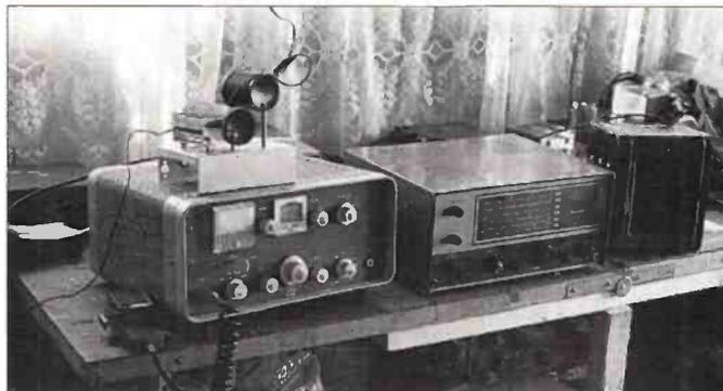
**Using the Heathkit RA-1 with a KW Vespa as an amateur station.**
