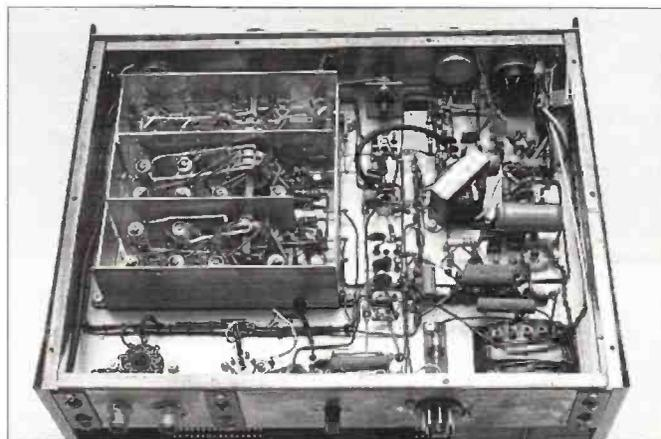
Internal view of the Heathkit RA-1, 6-band coil pack on left.
