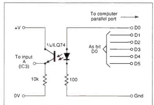
**Fig. 4: The complete circuit diagram of the interface.**
