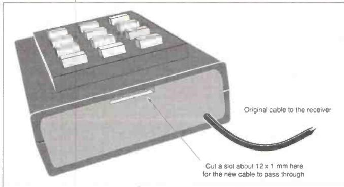
**Fig. 6:** The end of the keypad showing where to file the small notch needed to allow the ribbon cable to exit the box.
