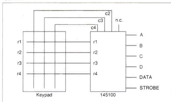
Fig. 2: Connecting the MC145100 in parallel with the keypad matrix.
