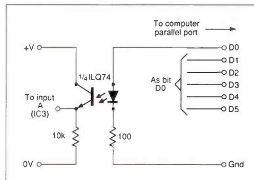
**Fig. 4: The complete circuit diagram of the interface.**
