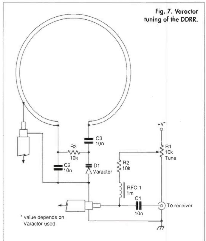
**Fig. 7. Varactor tuning of the DDRR.**
