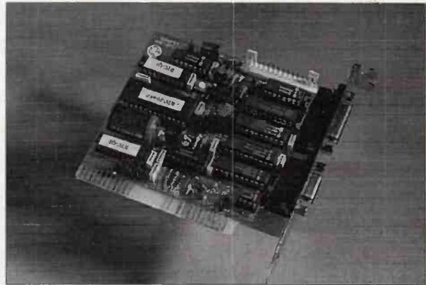
Sonifex announce their new Mentor MSF radio clock system, designed to ensure that your PC is synchronised to UK time automatically by utilising the broadcasts from the 60kHz l.w. Rugby MSF station. The signal from Rugby can be received in most UK locations.
