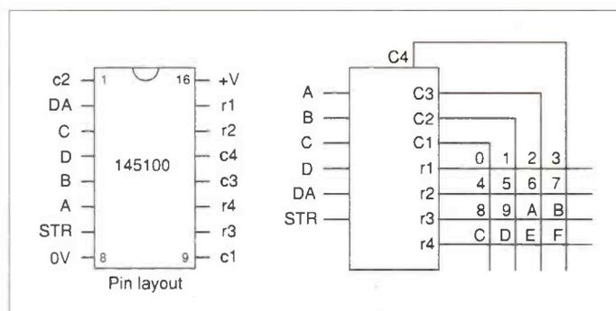
Fig. 1: The pin-out of the MC145100, showing how the 4x4 switch matrix appears.
