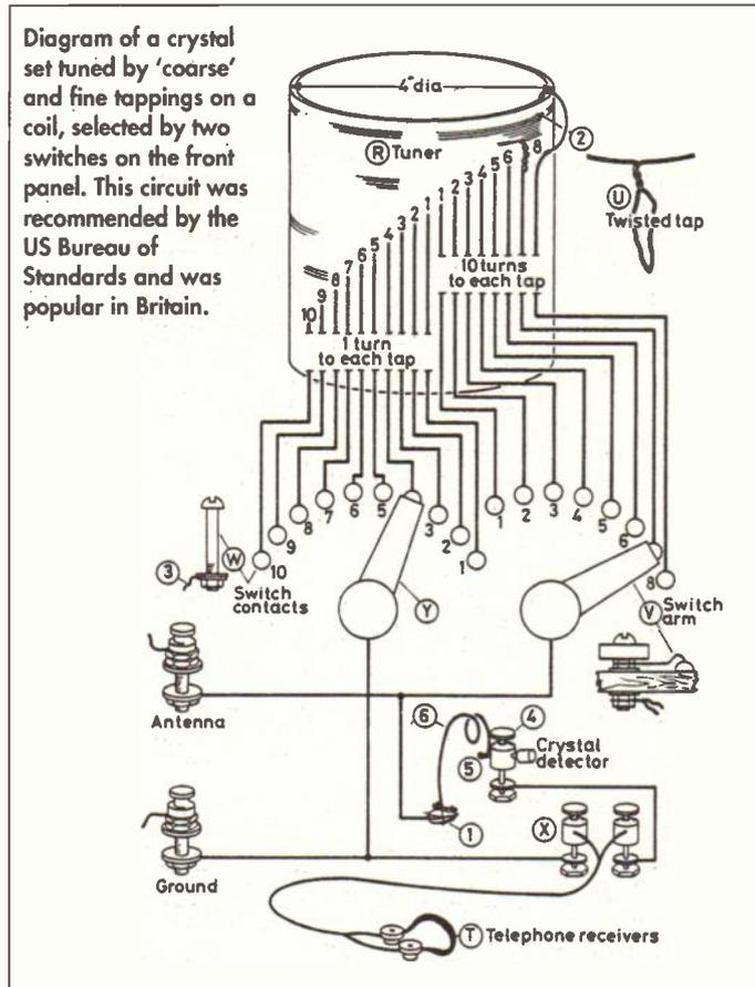
with a single earpiece. An alternative method was to buy a pair of cheaper 120Ω headphones and connect them by means of a suitable transformer to the output of the crystal set.
