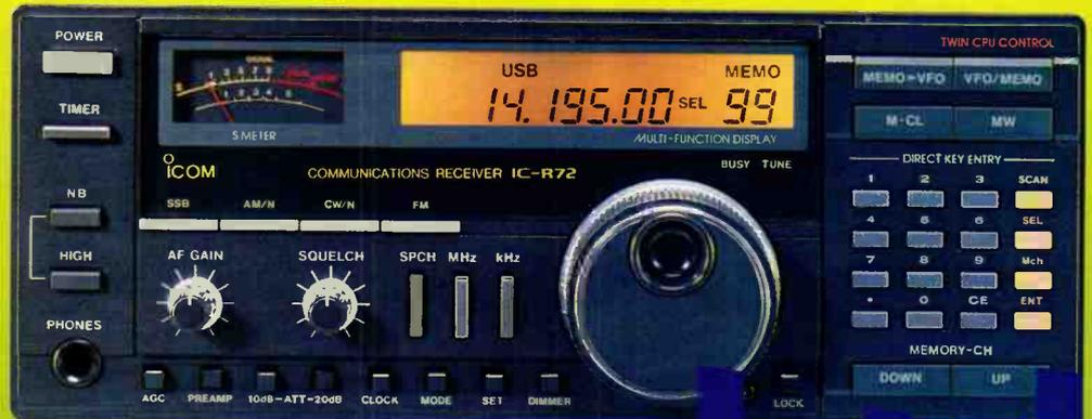
Shown above is ICOM's IC-R72 HF receiver, ideal for monitoring broadcasts, marine vessels, aircraft and emergency services on AM, SSB, CW plus optional FM between 100kHz and 30MHz. The IC-R72 has high sensitivity, an advanced DDS system, 100dB dynamic range and a very interesting range of options, as does the IC-R7100...
