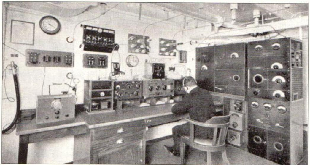
Typical 1930s Marconi passenger ship installation showing 2kW CW/ICW long wave transmitter type 388/387/389 and antenna distribution switches. On the desk can be seen 250W QG emergency transmitter and type 352A and 521 receivers. The receiver on the extreme left is used for broadcast reception.
