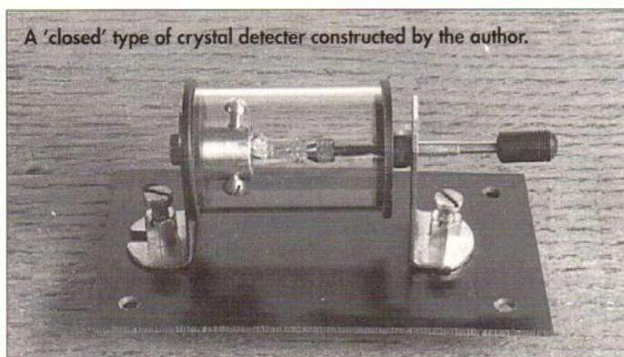
A 'closed' type of crystal detector constructed by the author.
