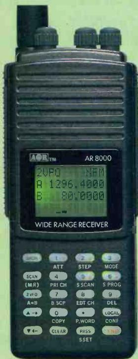
The **AR8000 UK** receiver is without doubt the most full featured wide band hand held receiver on the market today. Frequency coverage is from 500 kHz - 1900 MHz without gaps and all mode reception NFM, WFM, AM, USB, LSB & CW. The display provides twin frequency readout and alphanumeric comments for memory and search banks. The receiver may also be operated via computer using the optional CU8232 interface. The AR8000 UK is a remarkable receiver and a new concept in design.
