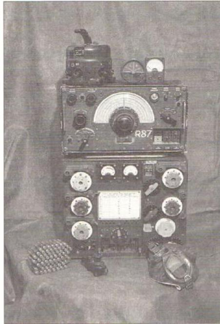
**The R1155/T1154 combination. The receiver is on top, along with the 'J' aerial switch (round object on top) and 'bathtub' Morse key. This was complete with locking ring that would hold set on transmit while aircrew bailed out of a stricken aircraft.**
