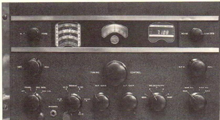
**A very good example of the trusty AR88D from RCA. This one, however, features a digital frequency display definitely not from WWII!**
