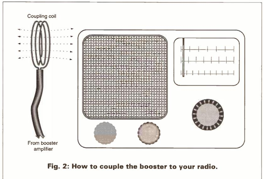
Fig. 2: How to couple the booster to your radio.
