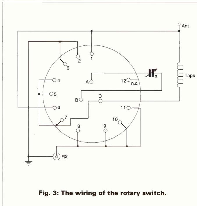
**Fig. 3: The wiring of the rotary switch.**
