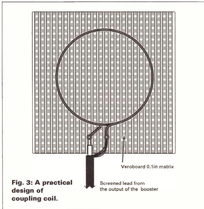
**Fig. 3: A practical design of coupling coil.**
