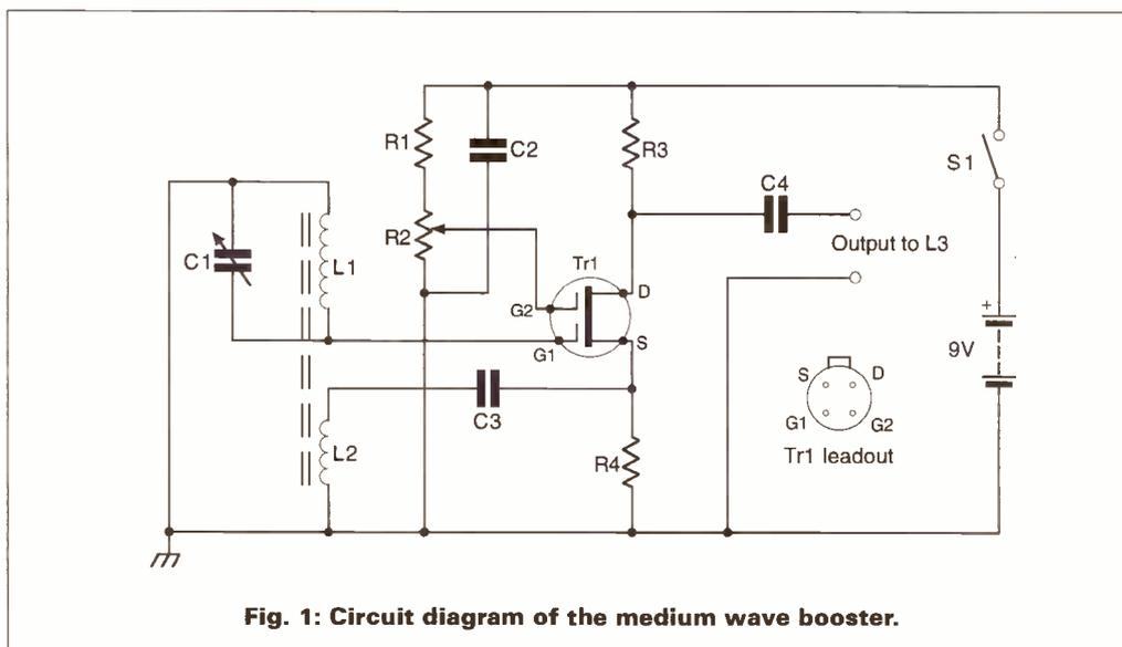
Fig. 1: Circuit diagram of the medium wave booster.
