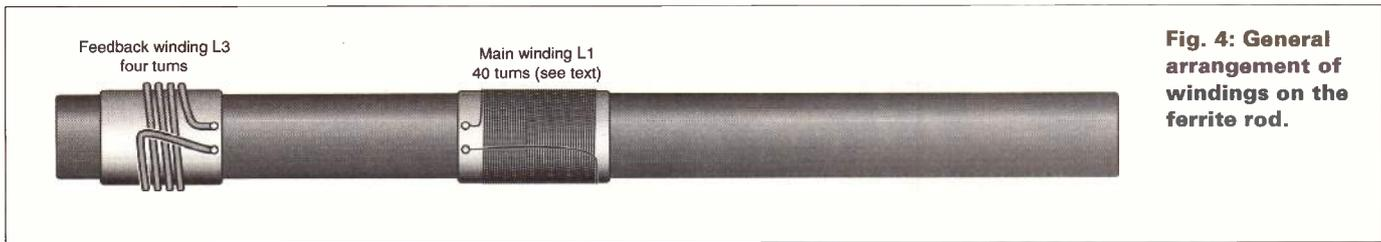
**Fig. 4: General arrangement of windings on the ferrite rod.**
