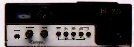
lowest long wave channel to the very top of the short wave band and the model's features include 30 memory channels, different filters to alter the bandwidth, synchronous detection and different operational modes for listening to different types of signals (like radio amateur transmissions). It performs superbly and comes highly recommended by experts in the field who note the no-frills design and easy to use controls.
