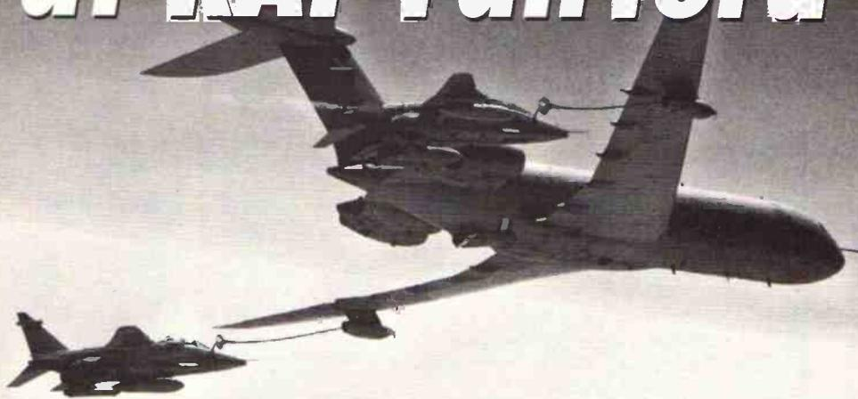
**An RAF VC-10 tanker refuels two Jaguars in flight.** Crown Copyright.
