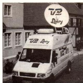
A typical SNG uplink truck, this the Danish TV2/Lorry mobile facility using Advent equipment built into a standard Iyeco 59.12 vehicle.
