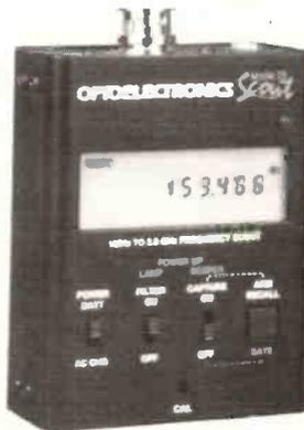
Of particular interest to operators of the AR2700 & AR8000 is the ability to connect the **Scout** directly to the receiver (small modification required) so that active frequencies are automatically fed to the AOR receiver which immediately jumps to the active frequency reported by the **Scout**, this feature is called **REACTION TUNE**. **Scout £399**
