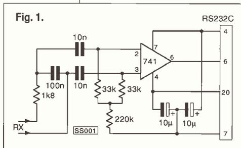
using portable receivers for utility monitoring. **Gordon West** of Olney has written this month with just such a suggestion. His design, see **Fig. 1**, uses the balanced input of a 741 Op-Amp to create a new interface.
