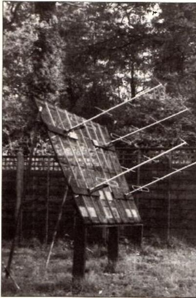
**Fig. 3: Ron Ham's radio telescope antenna array.**
