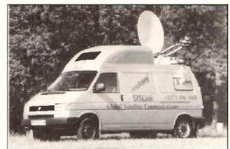
A SISLink satellite digital uplink truck used for SNG and general EFP work, this based on a VW Transporter chassis. (courtesy Francis, SISLink).
