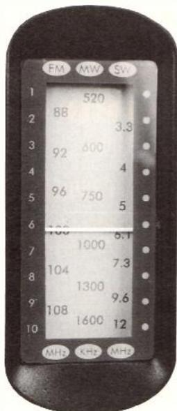
The simple dial. Backlash in the tuning system made tuning weak signals tricky.
