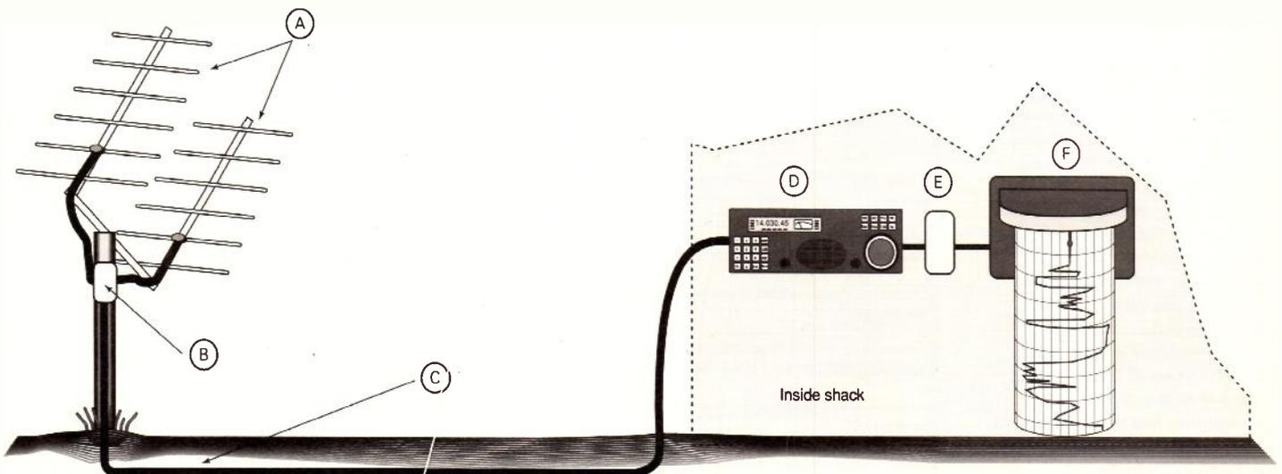
**Fig. 2: The layout of the radio telescope.**
