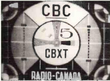
**A distinctive test card used until the early seventies by Canadian TV. The call sign and channel number were included in the centre. This example was radiated in the Edmonton area. The transmitter had an e.r.p. of 318kW.**
