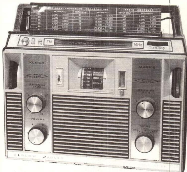
The Barlow Wadley XCR-30 Mk II receiver, showing the set tuned to 14.300MHz. Note the f.m. unit on top with the frequency chart also being displayed.
