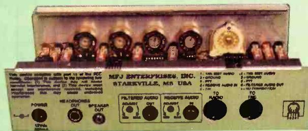
panel. A typical example of where this filter would be useful is to reduce interference from an adjacent station. If, for example, you were suffering a lot of high frequency splatter you could gradually wind-in the high frequency rejection to get the best compromise between signal readability and interference rejection.
