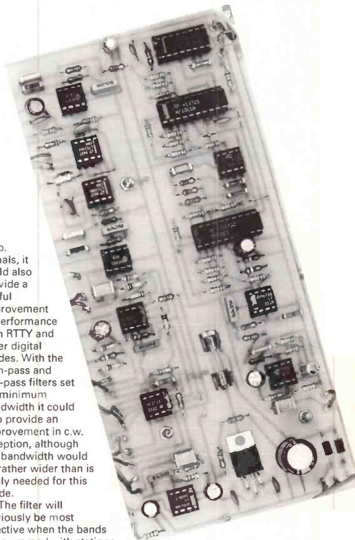
Completed printed circuit board.
