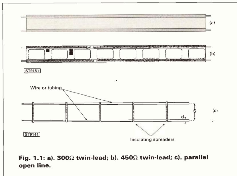
Fig. 1.1: a). 300Ω twin-lead; b). 450Ω twin-lead; c). parallel open line.
