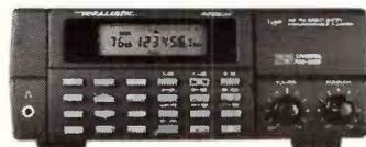
200 channels with Hyperscan system which lets you scan at 25 or 8 channels per second. High speed search facility locates new and unlisted frequencies at a flash. Coverage: 68-88, 108-136.975 (AM), 137-174, 380-512, 806-960MHz. This radio comes fitted with external aerial socket.
