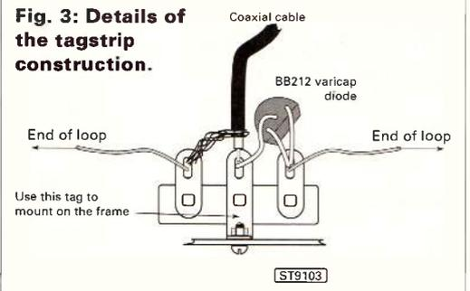
Fig. 3: Details of the tagstrip construction.
