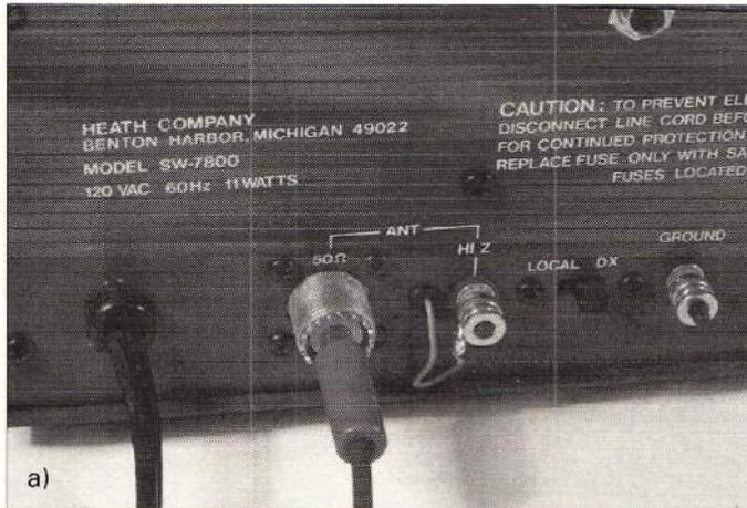
**Fig. 1.7: a) Connecting a single-wire downlead to a coaxial connector; b) Connecting a single wire to a coaxial cable - not recommended, but it works.**
