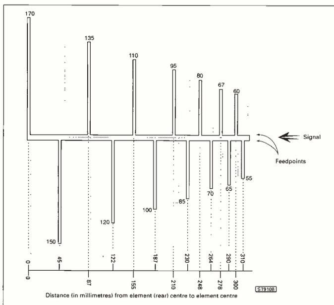
**Fig. 3:** The basic dimensions of the elements.
