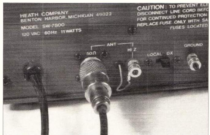
**Fig. 1.8: Coaxial cable to coaxial connector.**
