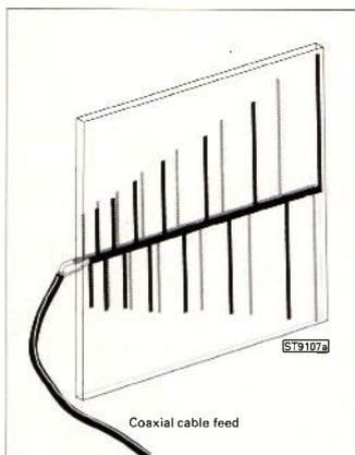
**Fig. 1:** The elements can be assembled on both sides of a single sheet of board.
