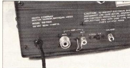
**Fig. 1.4:** Rear panel of a receiver showing both forms of connection.
