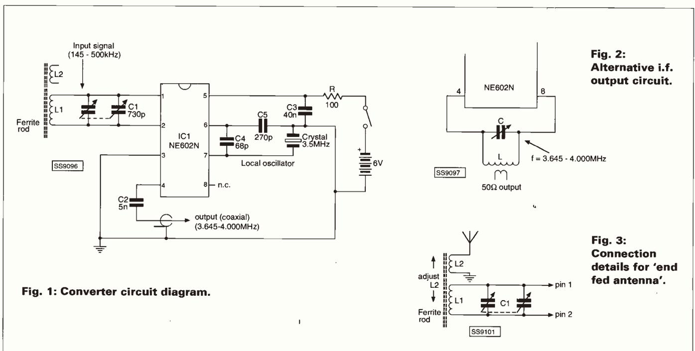
Fig. 1: Converter circuit diagram.
