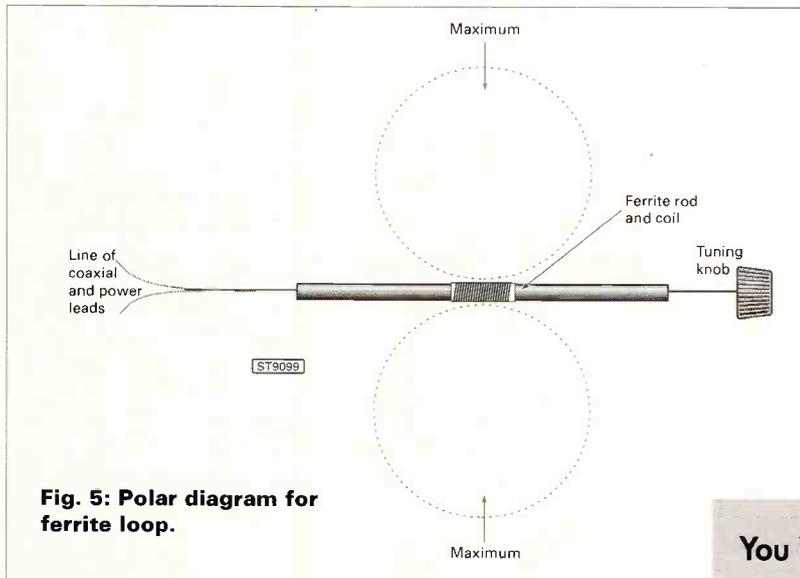
**Fig. 5: Polar diagram for ferrite loop.**
