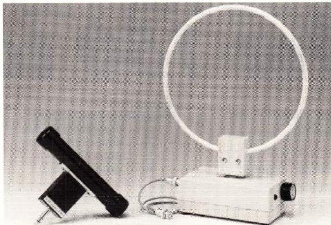
The aerial elements may be rotated in order to achieve maximum receive signal strength while minimising (nulling out) the effects of unwanted interfering local terrestrial signals. The vari-cap tuning featured in the LA320 also adds valuable selectivity to any receiver's front-end stages.
