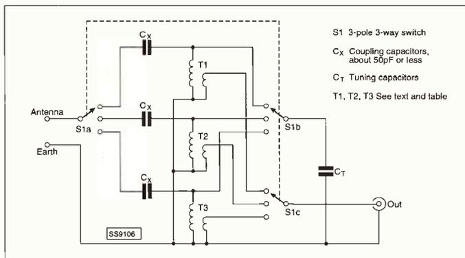
To connect the radio to the tuned circuit I use an extra small coil having about 20% of the turns of the main coil. The same criteria apply to this coil as apply to the coupling capacitor, the fewer turns the better. The coupling coil is wound at the earthy end of the tuning coil in between the other turns.
