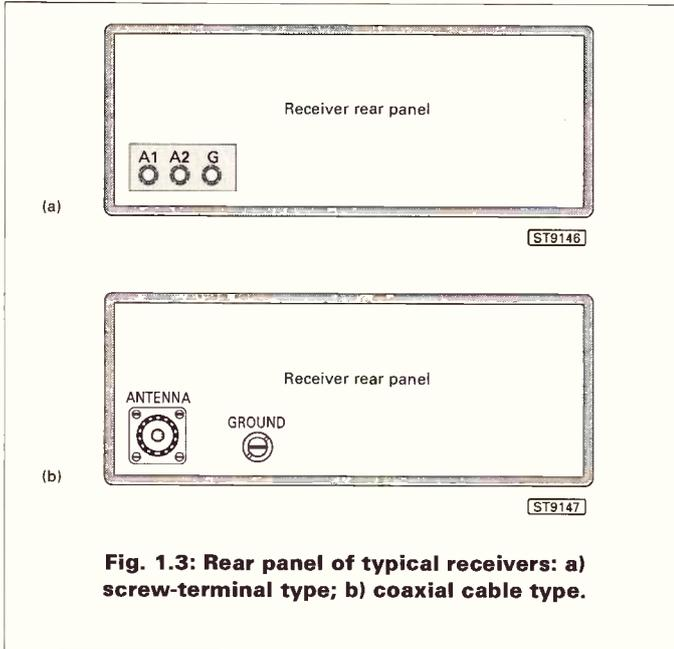
**Fig. 1.3:** Rear panel of typical receivers: a) screw-terminal type; b) coaxial cable type.
