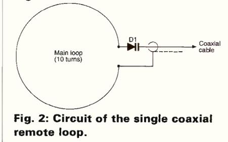
Fig. 2: Circuit of the single coaxial remote loop.
