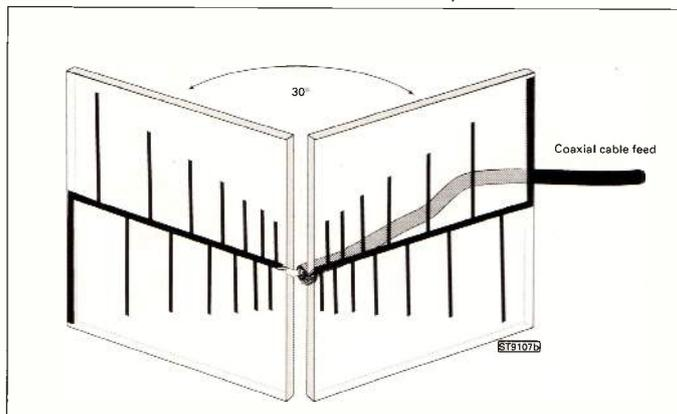
**Fig. 2:** Two separate single sided boards can be opened out at 30°.
