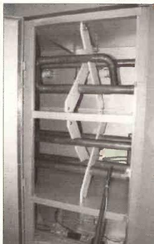
Shown here is one section of the anode inductor for the transmitter. Large diameter copper pipe is necessary because of the high power levels involved.
