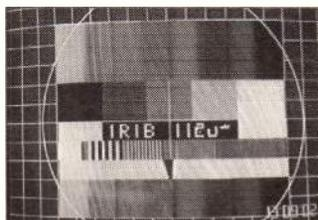
The Iran test card via Eutelsat II F4 at 7°E, stabilised with an EBU sound in sync (SIS) decoder.
