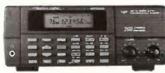
200 channels with Hyperscan system which lets you scan at 25 or 8 channels per second. High speed search facility locates new and unlisted frequencies at a flash. Coverage: 68-88, 108-136.975 (AM), 137-174, 380-512, 806-960MHz. This radio comes fitted with external aerial socket.
