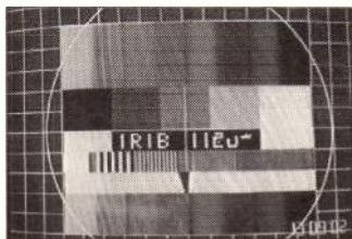
The Iran test card via Eutelsat II F4 at 7°E, stabilised with an EBU sound in sync (SIS) decoder.
