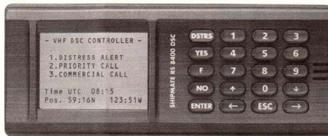
**A fixed combined v.h.f. DSC radio. Courtesy of SIMRAD Shipmate AS**
