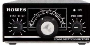
band modules. One module is provided with the kit (80m as standard, or to customers choice). Optional modules are available to cover all the h.f. amateur bands, 160 to 10m. Modules for other h.f. frequencies can also be used.
