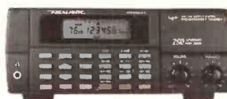
200 channels with Hyperscan system which lets you scan at 25 or 8 channels per second. High speed search facility locates new and unlisted frequencies at a flash. Coverage: 68-88, 108-136.975 (AM), 137-174, 380-512, 806-960MHz. This radio comes fitted with external aerial socket.
