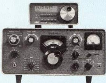
and spurious responses will occur. The v.f.o. tuning range is 2.695 to 2.495MHz which is below the normal operating frequency range of the transceiver, but the second harmonic is 5.390 to 4.990MHz whilst the third (although not mentioned by Collins) tunes 8.085 to 7.485MHz. The reason for quoting the frequencies tuning high to low is that due to the system configuration in the KWM-2 or 75S, the v.f.o. tunes 'backwards'.
