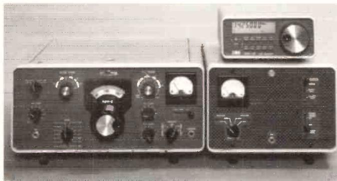
The DDS-2A from AOR is a microprocessor-controlled external VFO for the Collins KWM-2(A) and S-Line, including 75S-3B and 32S-3. The DDS-2A uses the latest DDS and PLL technology to produce accurate and clean local signal injections for the Collins radio.
