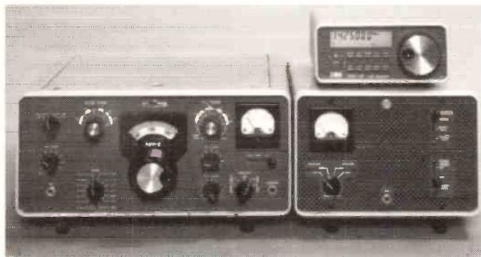
The DDS-2A from AOR is a microprocessor-controlled external VFO for the Collins KWM-2(A) and S-Line, including 75S-3B and 32S-3. The DDS-2A uses the latest DDS and PLL technology to produce accurate and clean local signal injections for the Collins radio.
