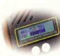
•Two-Line LCD display, first line displays frequency. Second line switches between either CTCSS, DCS, DTMF, Signal Strength, or Numerical Deviation.
