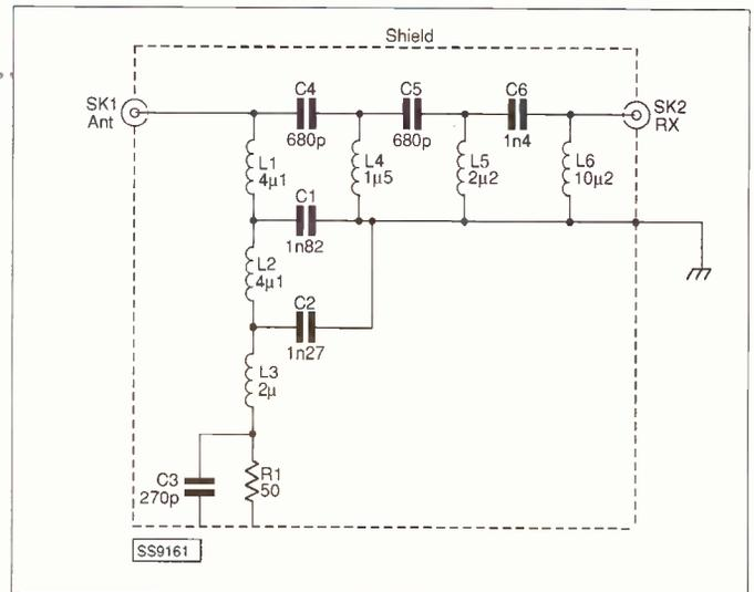
octave above  $F_c$ , -40+dB at two octaves and -60dB at three octaves. For a 3MHz signal, one octave is 6MHz, two octaves are 12MHz and three octaves are 24MHz. My results were slightly less than these figures because some of my components were ill-matched (e.g. slug-tuned commercial inductors were used rather than toroidal core coils), but the results were consistent with expectations.
