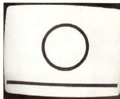
**One of the earliest test charts to be radiated by the BBC. This check for correct picture ratio was transmitted in 1934 using Baird's 30-line system - some two years before the start of high-definition television.**
