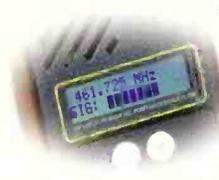
*•Two-Line LCD display, first line displays frequency. Second line switches between either CTCSS, DCS, DTMF, Signal Strength, or Numerical Deviation.*
