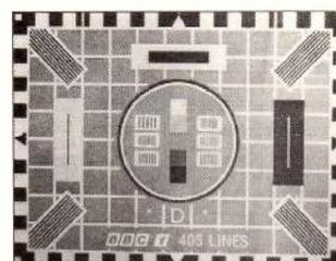
Fig. 7: The BBC-1 Test Card 'D' was introduced on April 20th, 1964 to mark the start of BBC-2 on u.h.f. 625-lines.
