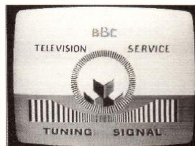
**A BBC Tuning Signal radiated in 1937. It was transmitted several minutes before the start of programmes to give the valved receivers time to 'warm up'!**
