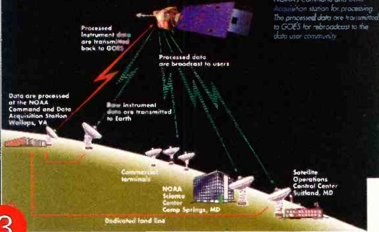
Instruments on board GOES scan the Earth for information and transmit their observations to NOAA's Command and Data Acquisition station for processing. The processed data are transmitted to GOES for rebroadcast to the data user community.
