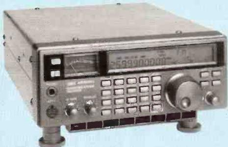
New high performance base / mobile wide band receiver offering great sensitivity and **excellent strong signal handling**. The AR5000 is housed in a newly designed **solid metal cabinet** and provides a very wide receive frequency coverage from **10kHz to 2600MHz, all mode reception** FM, AM, USB, LSB & CW and MANY microprocessor facilities aimed toward professional monitoring and the dedicated listener.
