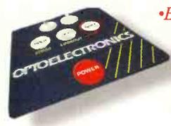
*•Easy touch control pad. F1 & F2 keys control all Xplorer functions. Hold, Skip, Store and Lockout all enabled through the keypad.*
