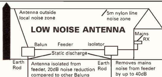
**UNIVERSAL MAGNETIC BALUN** • Match Longwire, dipole, T2FD to receiver • Unique design • 100kHz-30MHz. **EACH**
