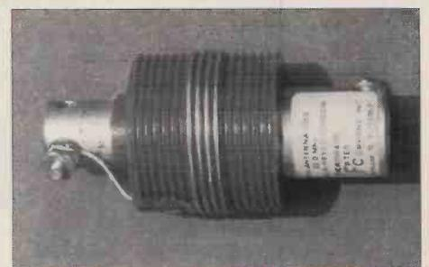
**Fig. 3:** A dipole tuning capacitor by Heathkit (still occasionally seen on sale at hamfests and rallies).
