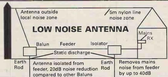
UMB 130 ● 10:1 BALUN for T2FD, LONGWIRE ● Isolated feeder winding rejects noise ● 100kHz-30MHz.
