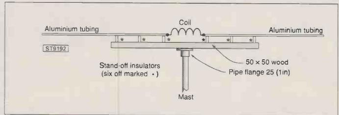
**Fig. 5: Construction details of a coil loaded rotatable dipole.**
