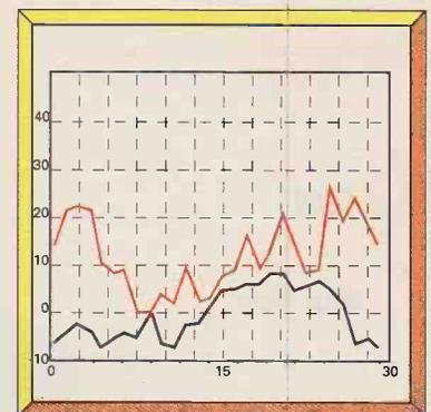
**Plot of 14MHz score for February against solar flux. Better correlation but the band conditions were dominated by the unsettled geomagnetic field so this is not a good comparison. Note how the solar flux was very steady in February compared with the fluctuations in January.**
