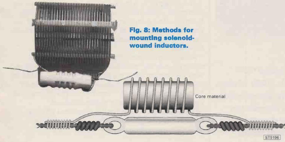
**Fig. 8: Methods for mounting solenoid-wound inductors.**
