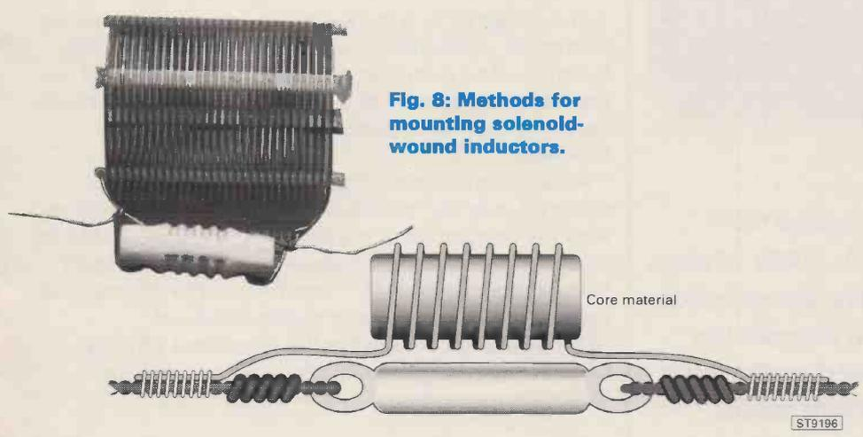
**Fig. 8: Methods for mounting solenoid-wound inductors.**
