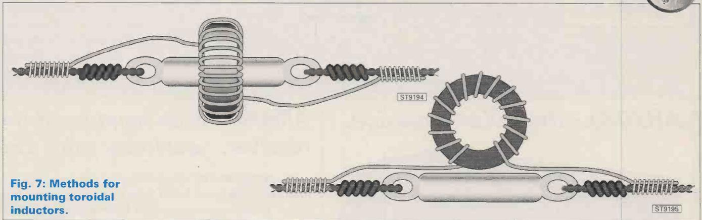
**Fig. 7: Methods for mounting toroidal inductors.**
