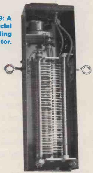
**Fig. 9: A commercial loading inductor.**
