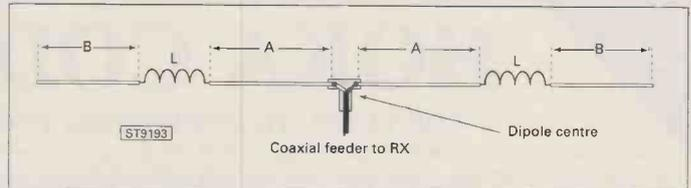
**Fig. 6: Two-coil loaded, shortened dipole.**
