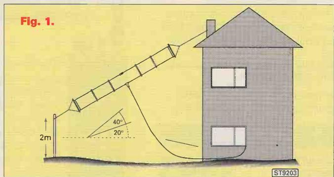
at the far end of the garden. The dipole is fed half way along one side, with the other side split at the half way point and a non inductive terminating resistor inserted as shown in **Fig. 2**. The performance of the T2FD, in my experience, is very much decided by the method of feeding it and the value of the termination resistor, and they are both critical (see **Fig. 1**).
