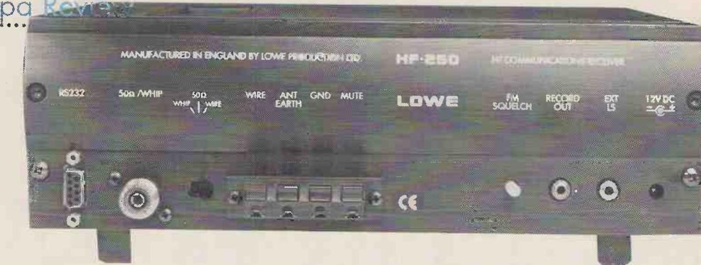
strong signal performance. Lowe receivers have always produced good audio quality and the HF-250 uses a full wave envelope detector for a.m. and a product detector for s.s.b. and c.w. There is also a fully automated noise blanker system that operates on the recovered audio.
