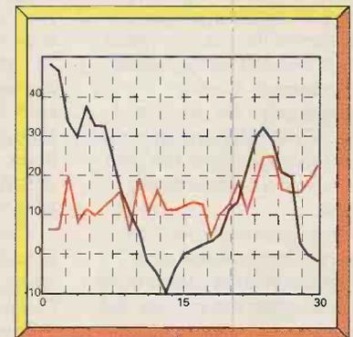
**The 14MHz score for January plotted against the 2.8GHz solar flux. The solar flux curve has been equalised with the 14MHz score by deducting 100 from the flux value. There is little correlation except in the last week of the month, but I believe the effects were masked by geomagnetic disturbances.**
