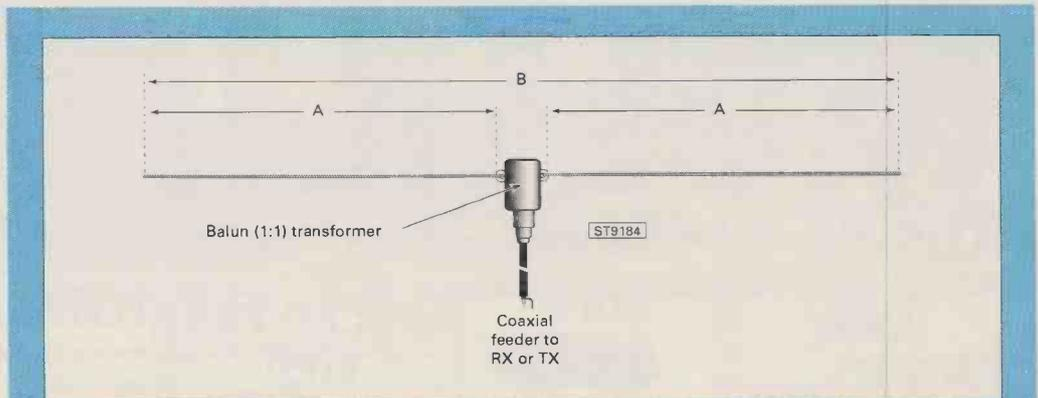
**Fig. 1:** A) Half-wavelength standard dipole; B) idealised dipole azimuthal (seen from above) pattern.
