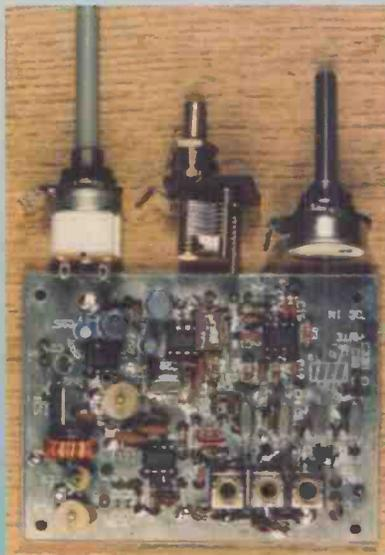
**The Hands Electronic RX1 superhet receiver. This is the completed printed circuit board awaiting testing and alignment before being fitted into a case. The RX1 p.c.b. is quite densely packed and needs a steady hand on the soldering iron**
