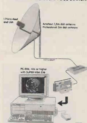
Fig.5: Diagram of a PC-based NOAA-h.r.p.t. receiving system - from Martin Duinen.
