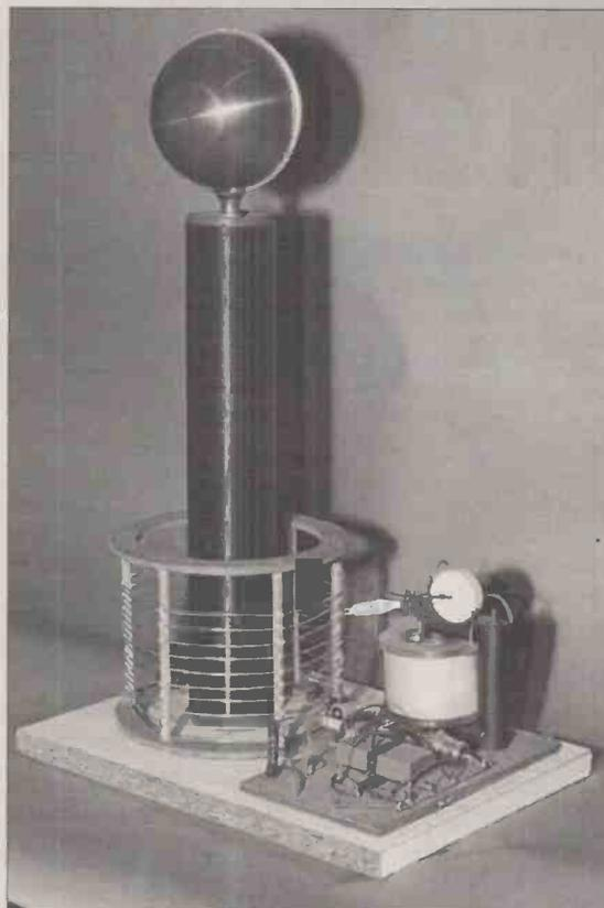
**This is the larger of C.M. Lindars' two Tesla coils. The copper ball was originally intended to be a vital piece of household plumbing!**
