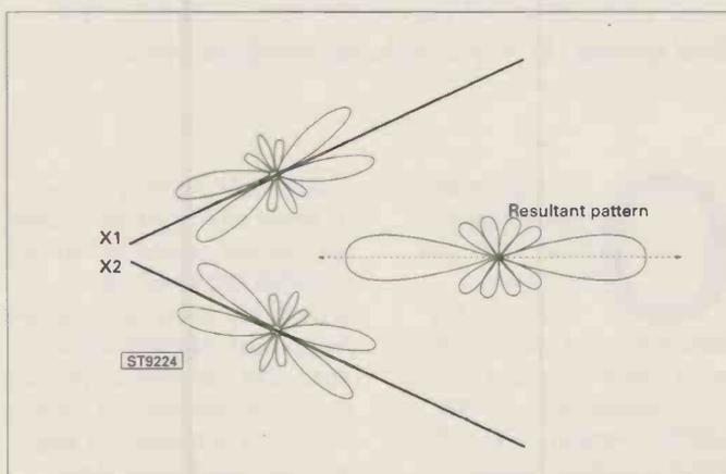
**Fig. 4: The basic resonant Vee-beam antenna.**
