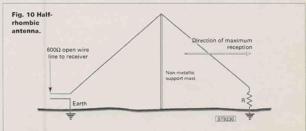
Fig. 10 Half-rhombic antenna.
