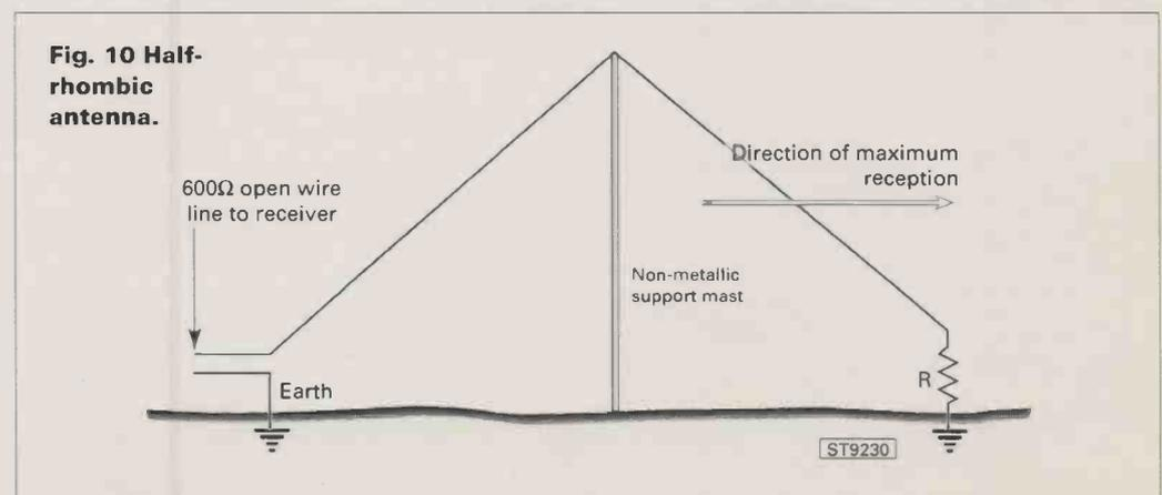
Fig. 10 Half-rhombic antenna.
