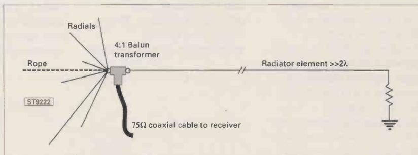
**Fig. 2: The non-resonant, terminated long-wire.**
