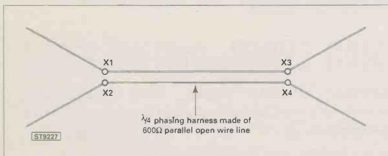
Fig. 7 Stacking Vee-beams gives 3dB more gain.
