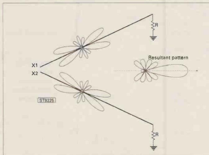
**Fig. 5: The non-resonant Vee-beam antenna.**
