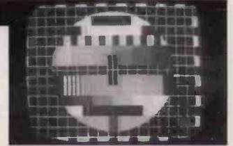
**Fig. 1:** A rare sight these days! TVP-1 Poland using the PM5544 with a dark-background. High-power Band I transmitters are no
