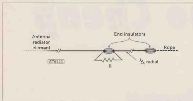
**Fig. 3: Method of using a counterpoise ground with the terminating resistor.**
