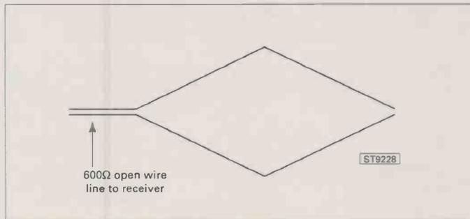
Fig. 8 Resonant rhombic antenna.
