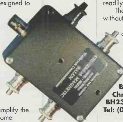
simplify the home construction of the T2FD antenna. A specially wound 9:1 Balun, together with a thick film 500Ω 5W termination resistor, is fitted into a small ABS box. The completed assembly is encapsulated in epoxy resin to ensure reliability in the most severe weather conditions.
