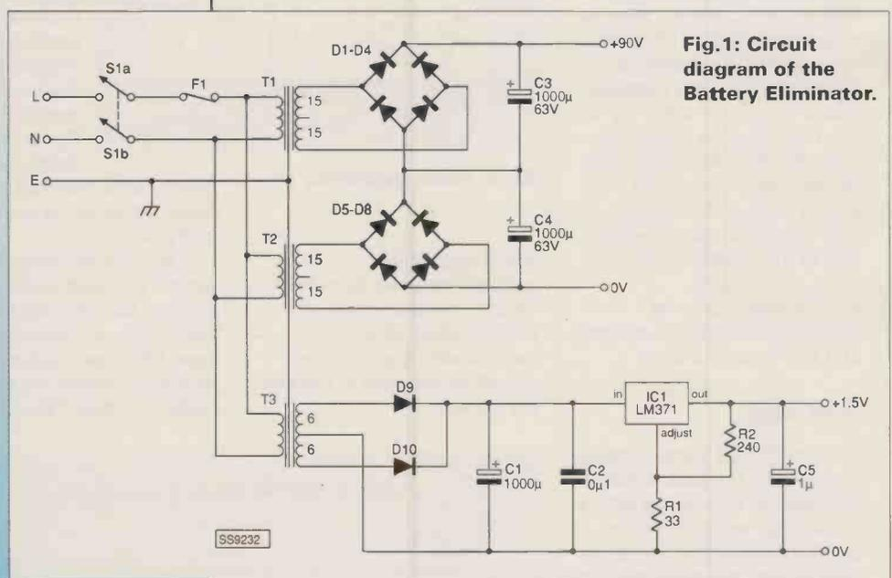
**Fig. 1: Circuit diagram of the Battery Eliminator.**
