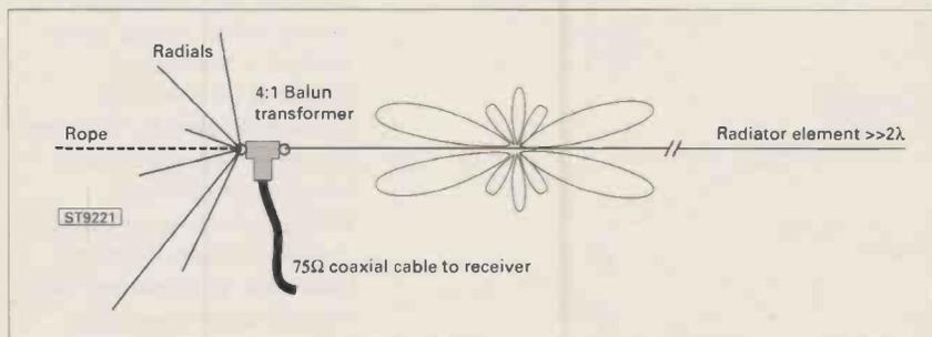
**Fig. 1: The basic resonant (unterminated) long-wire antenna.**
