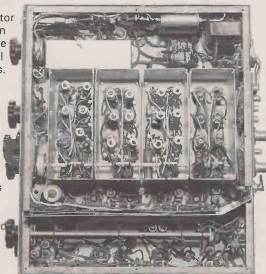
They don't build 'em like this any more. The underside wiring of the CR100/2.
