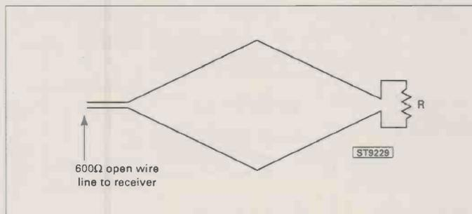
Fig. 9 Non-resonant rhombic antenna.
