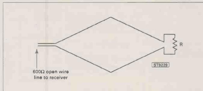
Fig. 9 Non-resonant rhombic antenna.
