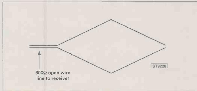
Fig. 8 Resonant rhombic antenna.
