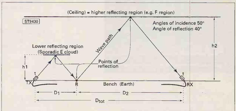
(e) are multiples from a simulated sporadic E cloud (as in Fig. 2.5), whilst (f1) and (f2) are primary and secondary from the simulated F region (ceiling).
