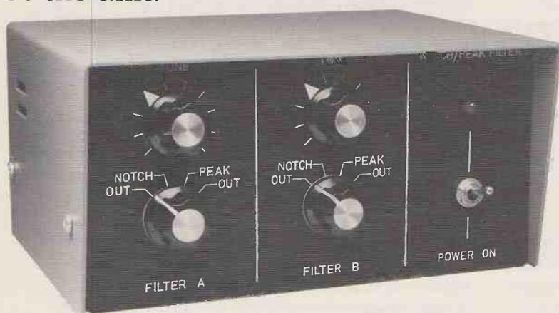
**C**onstruction of the filter is quite straightforward using a piece of Veroboard on which to mount the components and placing the potentiometer and rotary switch on the front panel of a suitable instrument case. The arrangement of the components and the positions where the tracks have to be cut is shown in Fig. 2.1. The layout shown is for two filters, but readers who are interested in constructing only a single filter, should ignore Filter A and start their board at track 13.
