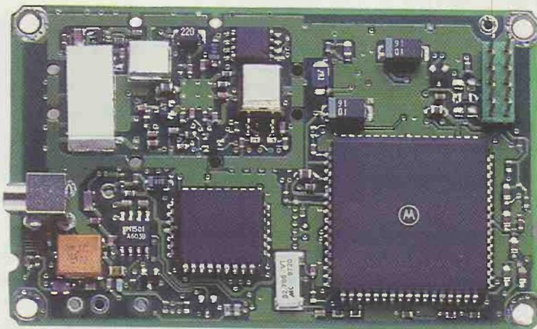
*New features on the UT Plus Oncore GPS from Motorola give the receiver greater immunity from unintentional jamming.*
