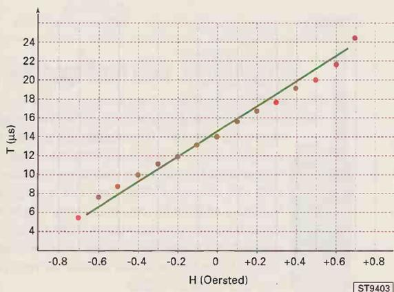
another. This orthogonal arrangement permits easier implementation of orientation measurement, compass and other applications. The FGM-3h is the same size and shape as the FGM-3, but is about 2.5 times more sensitive. The output frequency changes approximately 2 to 3Hz per gamma of field change, with a dynamic range of 0.15oersted (about one-third the earth's magnetic field strength).
