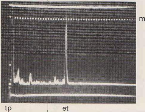
Fig. 2.9: Photo from oscilloscope. Simulation of OTH radar. (tp) transmitter pulse; (et) echo from target located near earth (bench) at a surface distance of 2.24m; (m) 1ms markers (see text).
