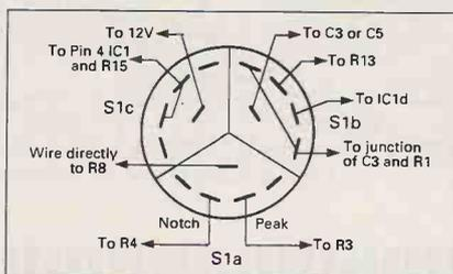
Fig. 2.2: Revised version of rotary switch S1. One of these is required for each filter section.
