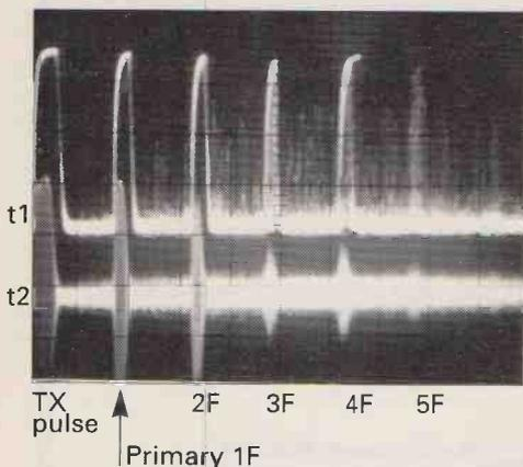
Fig. 2.1: Real primary and multiple echoes from the F region. Frequency 6.5MHz, p.r.f. 35Hz, pulse width 0.75ms.
