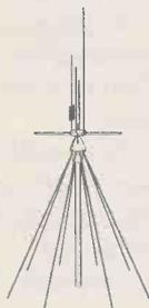
**Skyscan DX-V1300 base disconn** – Most disconnes only have horizontal elements and this is the reason that they are not ideal for use with a scanner. Most of the transmissions that you are likely to receive on your scanner are transmitted from vertically mounted antennas. The DX-V1300 has both vertical and horizontal elements for maximum reception. Constructed from best quality stainless steel and aluminium and comes complete with mounting pole. **£49.95** + £3 P&P.
