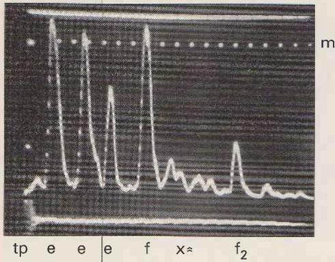
Fig. 2.6: Photo from oscilloscope. Simulation of 'N' mode propagation (tp) transmitted pulse. (e,e,e) pseudo sporadic E primary and two multiple echoes (f, f<sub>2</sub>) pseudo F region primary and one multiple echo (x) small spurious echoes (see text); (m) 1ms: markers.
