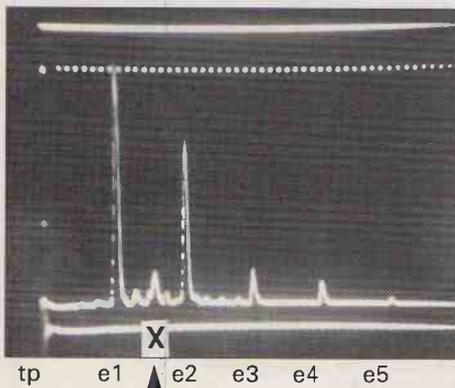
Fig. 2.2: Indoor simulation with ultrasonics of multiple echoes from a pseudo reflecting F region, i.e. the ceiling. Frequency 40kHz; p.r.f. 20Hz; pulse width 1ms; Markers (m) 1ms; (tp) transmitted pulses; (e1) primary echo; (e2, e3, e4, e5) multiple echoes; (x) see text.
