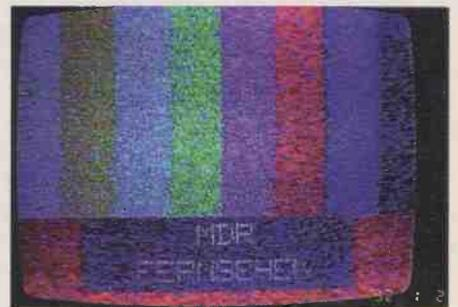
Fig. 2: German FuBK test card from MDR displaying local identification, circa 1992.
