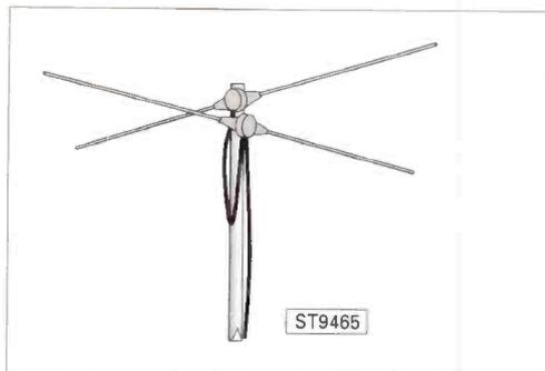
Fig. 7: Single-set crossed dipole.
