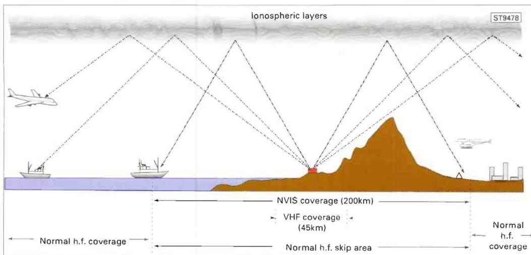
**Fig. 1: Near Vertical Incidence Skywave propagation. NVIS bridges the gap between the nominal v.h.f./u.h.f. coverage area and the typical h.f. 'skip zone'.**
