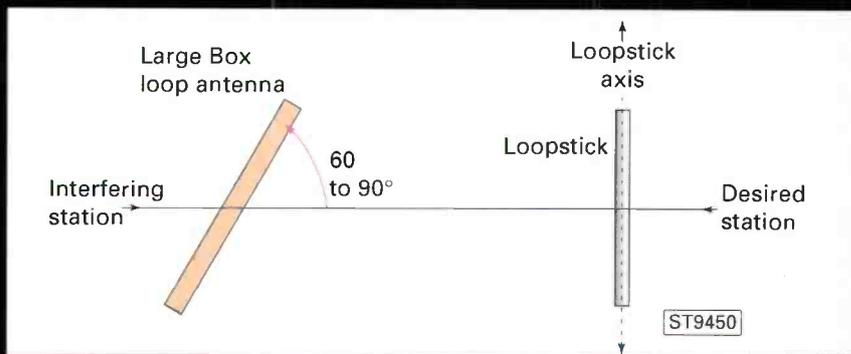
Fig. 2.1: Use of a spoiler loop to null, coaxial, same or adjacent channel interference.
