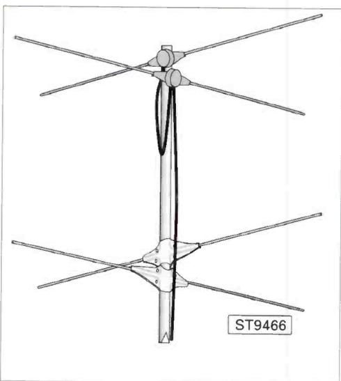
Fig. 8: Standard crossed-dipole.
