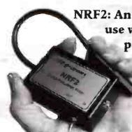
**NRF2:** An effective, yet realistically priced, audio filter for use with any receiver. Just plug it in to your headphone or speaker socket to reduce the hash whistles and splatter that hide your DX! This is a 'passive' device, with no need for batteries!
