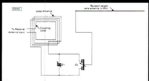
**Fig. 2.10: a) use of a differential capacitor for phasing and amplitude control; b) a differential capacitor.**
