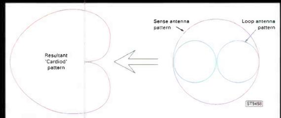
**Fig. 2.6: Combining figure-8 and omnidirectional patterns to produce the cardioid pattern.**
