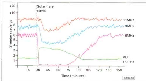
**Fig. 7: Typical strengths of broadcast signals before, during and after a SID. VLF signal enhancement is also shown.**
