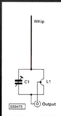
**Fig. 1: Circuit of matching transformer.**
