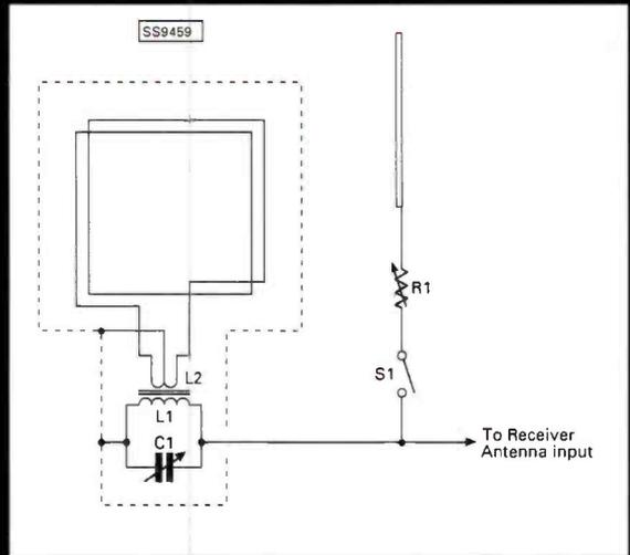
**Fig. 2.7: Use of a sense antenna to produce cardioid pattern.**
