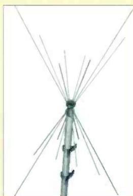
The Airmaster 117-137MHz and 224-400MHz airband antenna is a high performance, dedicated, civil and military airband antenna. Two pairs of angled dipoles cover the 117-137MHz civil band, and six pairs of angled dipoles cover the 224-400MHz military band nominal impedance is 50Ω via an N-type connector.
