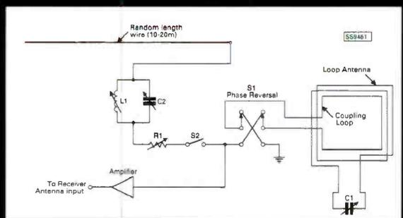
**Fig. 2.9: Adding phasing control to the random wire sense antenna.**
