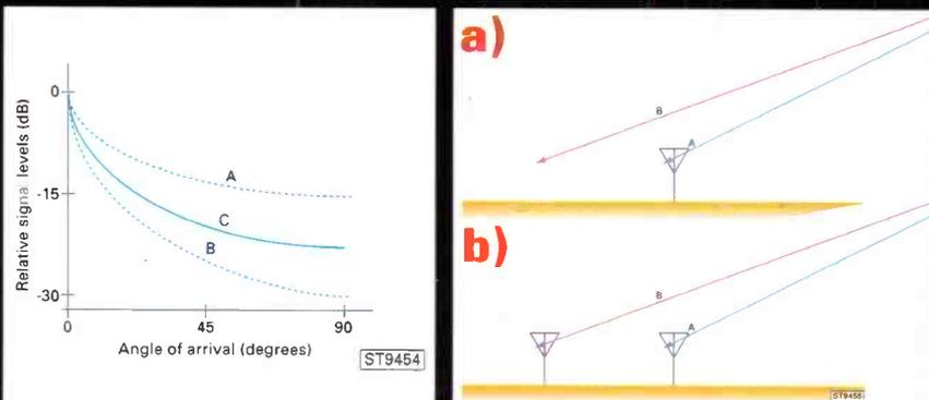
Fig. 2.3: Relative signal level v angle of arrival for three ground conditions.
