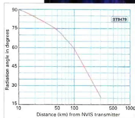
**Fig. 2: Graphical representation of the range in km from the NVIS site, versus elevation angle.**
