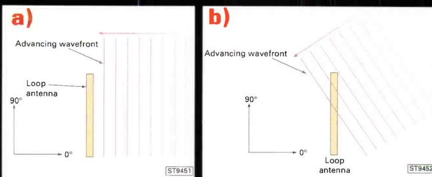
Fig. 2.2 a) 0° angle of arrival; b) 45° angle of arrival; c) 90° angle of arrival.
