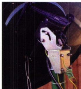
The horizon-to-horizon (h-to-h) motor on the back of my dish, exposed to the weather.
