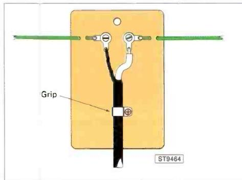
Fig. 6: Dipole connection.
