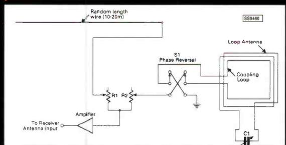
**Fig. 2.8: Use of a random length wire sense antenna.**
