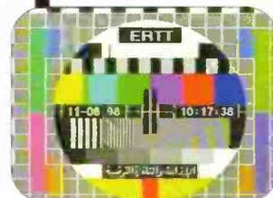
**Fig. 2: The Philips PM5534 test card transmitted by RTT, Tunisia.**
