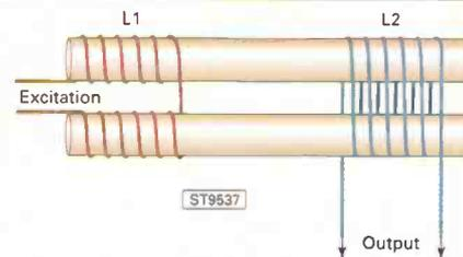
Fig. 3.7: Ferrite rod flux-gate magnetometer.
