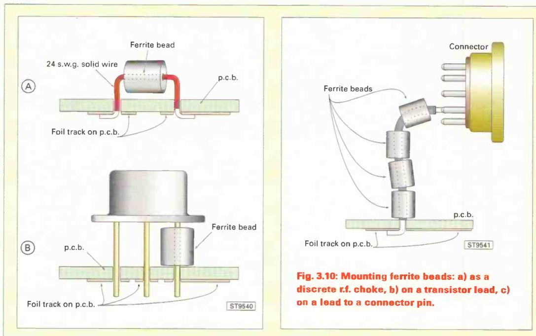
**Fig. 3.10: Mounting ferrite beads: a) as a discrete r.f. choke, b) on a transistor lead, c) on a lead to a connector pin.**
