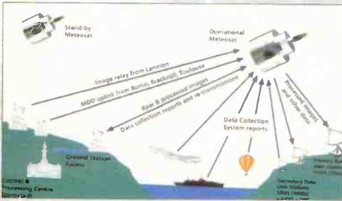
**Fig. 11: METEOSAT communications channels.**
