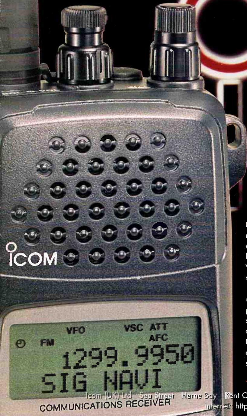
ICOM's great handheld receiver covers 0.5MHz-1300MHz in all-modes. The IC-R10 boasts a real-time bandscope function, making it easy to find busy frequencies and observe the receiving frequency band conditions, also, the passband width of the scope is selectable. Voice-scan function (VSC) pauses scan, but only when modulated signals are received.
