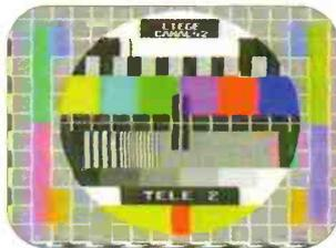
**Fig. 7:** The Philips PM5544 electronic-generated test card broadcast by the French-language TV service in Belgium.
