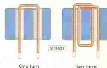
**Fig. 3.2: Turns counting in the binocular core: a) one-turn, b) two-turns.**
