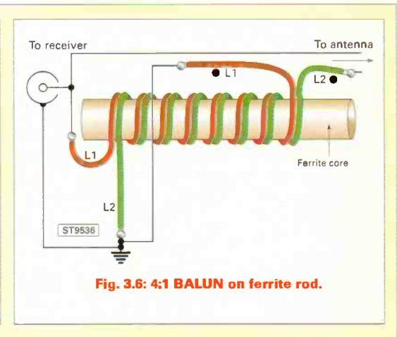
**Fig. 3.6: 4:1 BALUN on ferrite rod.**
