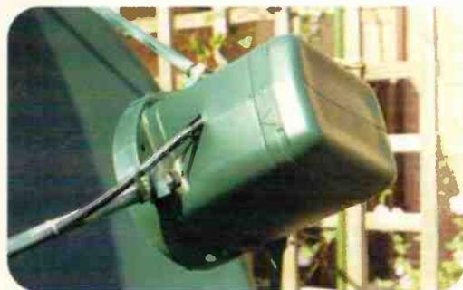
**Fig. 2:** The 4GHz LNB is protected with this cover made from a two litre polythene white spirit container.
