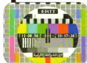
**Fig. 2: The Philips PM5534 test card transmitted by RTT, Tunisia.**
