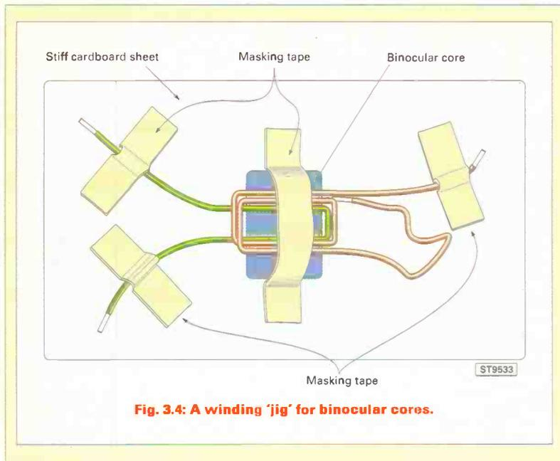
**Fig. 3.4: A winding 'jig' for binocular cores.**
