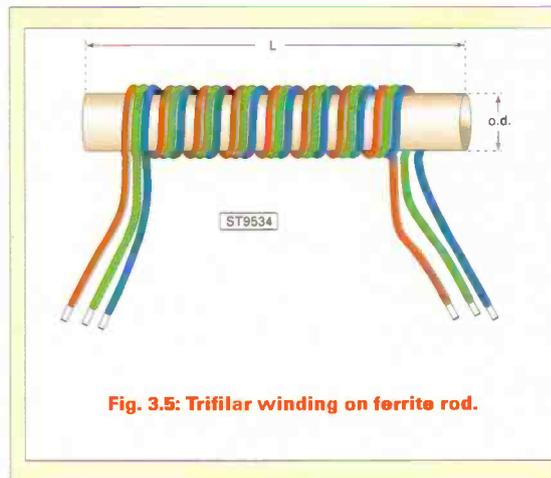
**Fig. 3.5: Trifilar winding on ferrite rod.**
