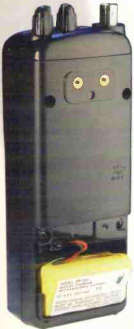
The plug-in heat shrink NiCad battery pack.
