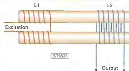
Fig. 3.7: Ferrite rod flux-gate magnetometer.
