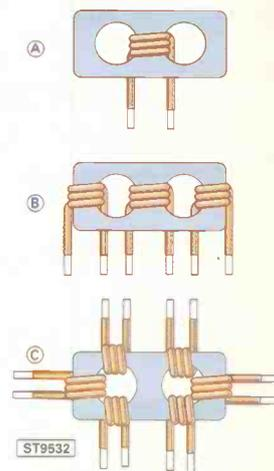
**Fig. 3.3: Winding styles for binocular cores (Fig. 3.3a preferred).**
