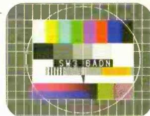
**Fig. 1: The FuBK electronically-generated test card radiated by Südwest-3 from Baden Baden, Germany.**
