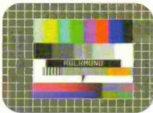
**Fig. 6:** The FuBK test card from the Dutch transmitter at Roermond, received in the UK during enhanced tropospheric conditions.
