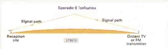
**Fig. 2: Television signals can be refracted back to earth by layers of ionised gases.**
