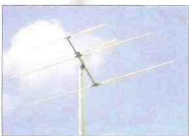
An antenna suitable for receiving Bands I and III DXTV signals.
