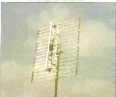
A wideband 'bowtie' array for u.h.f. DXing.
