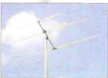
An antenna suitable for receiving Bands I and III DXTV signals.
