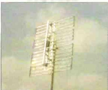
A wideband 'bowtie' array for u.h.f. DXing.
